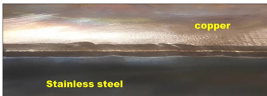
Figure 1. The appearances of the joints
