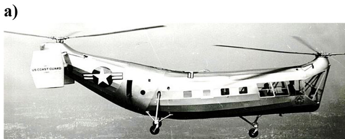
Figure 11. Production versions of tandem-rotorcraft helicopters: a) Piasecki HRP-1 [69]; b) McCulloch MC-4 [70]
