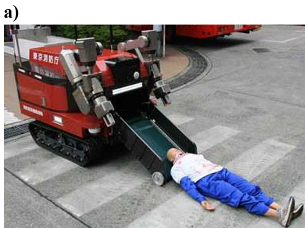
Figure 21. Mobile rescue robots: (a) RoboCue [104]; (b) Battlefield Extraction Assist Robot [105]
