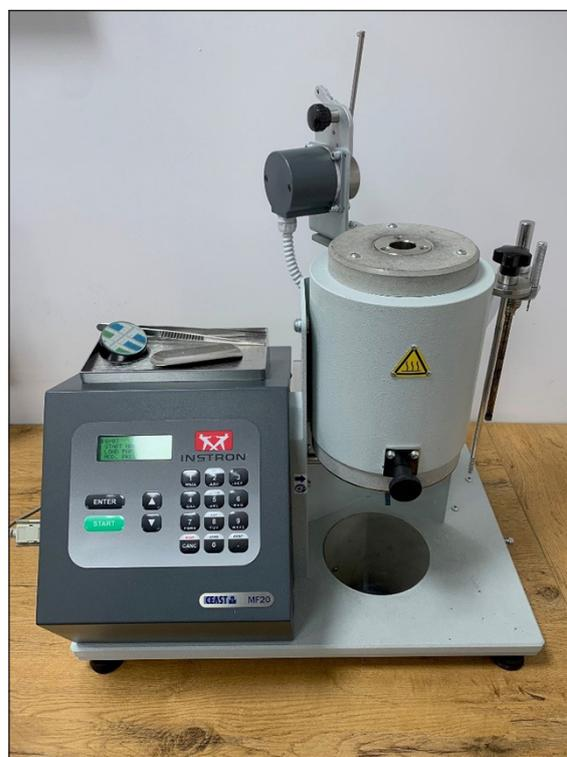
Fig. 2. General appearance of the CEAST MF20 Plastometer
