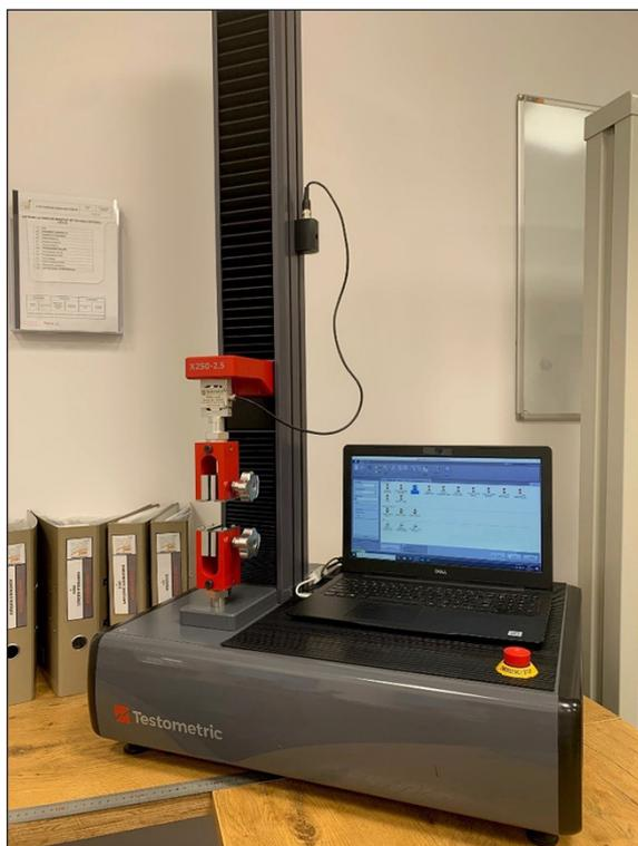
Fig. 4. General appearance of the Testometric X250-2.5 testing machine
