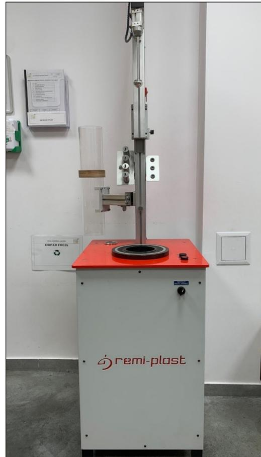
**Fig. 6.** General appearance of the device for measuring puncture resistance using the falling dart method
