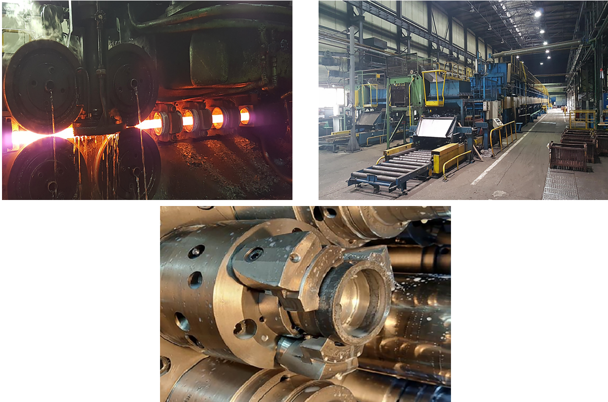
Figure 1. Preparation of bearing rings (from left): forging, annealing and turning
