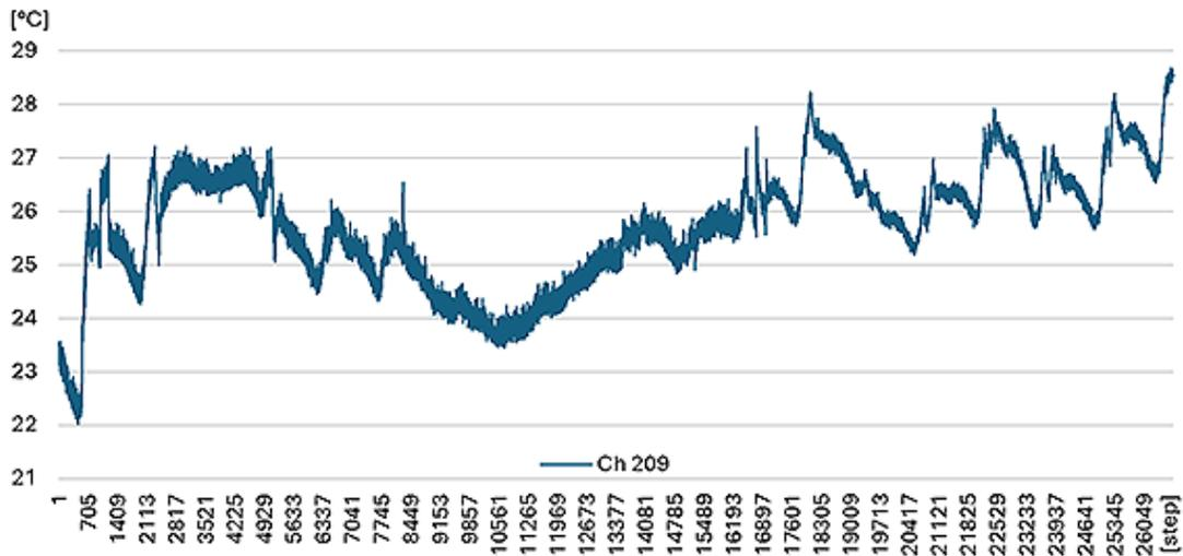
Figure 6. Temperature measurement profile (Ch209) on the internal side of the partition
