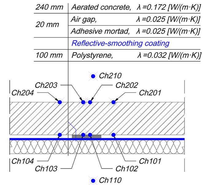
Figure 5. The distribution of temperature sensors in the analysed wall covered by the reflective-smoothing coating
