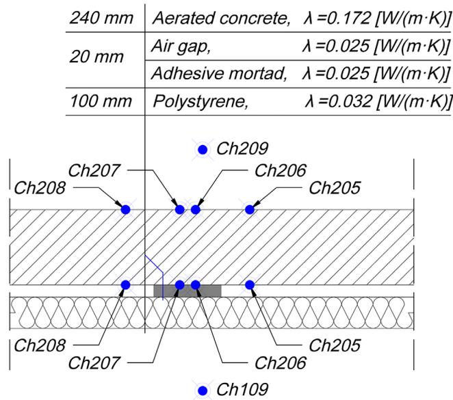
Figure 4. The distribution of temperature sensors in the analysed wall
