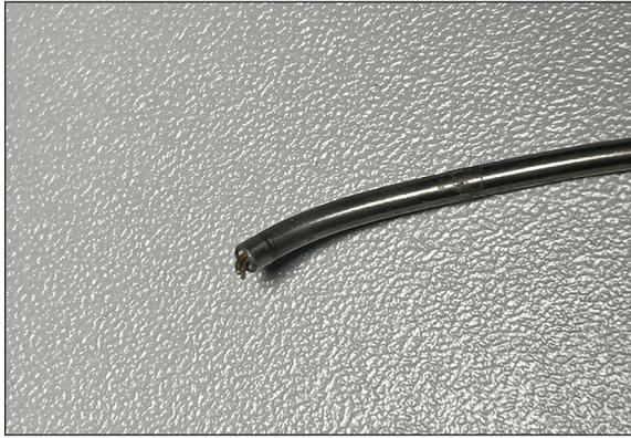
**Figure 8.** Defective, damaged during the experiment Pt100 temperature sensor
