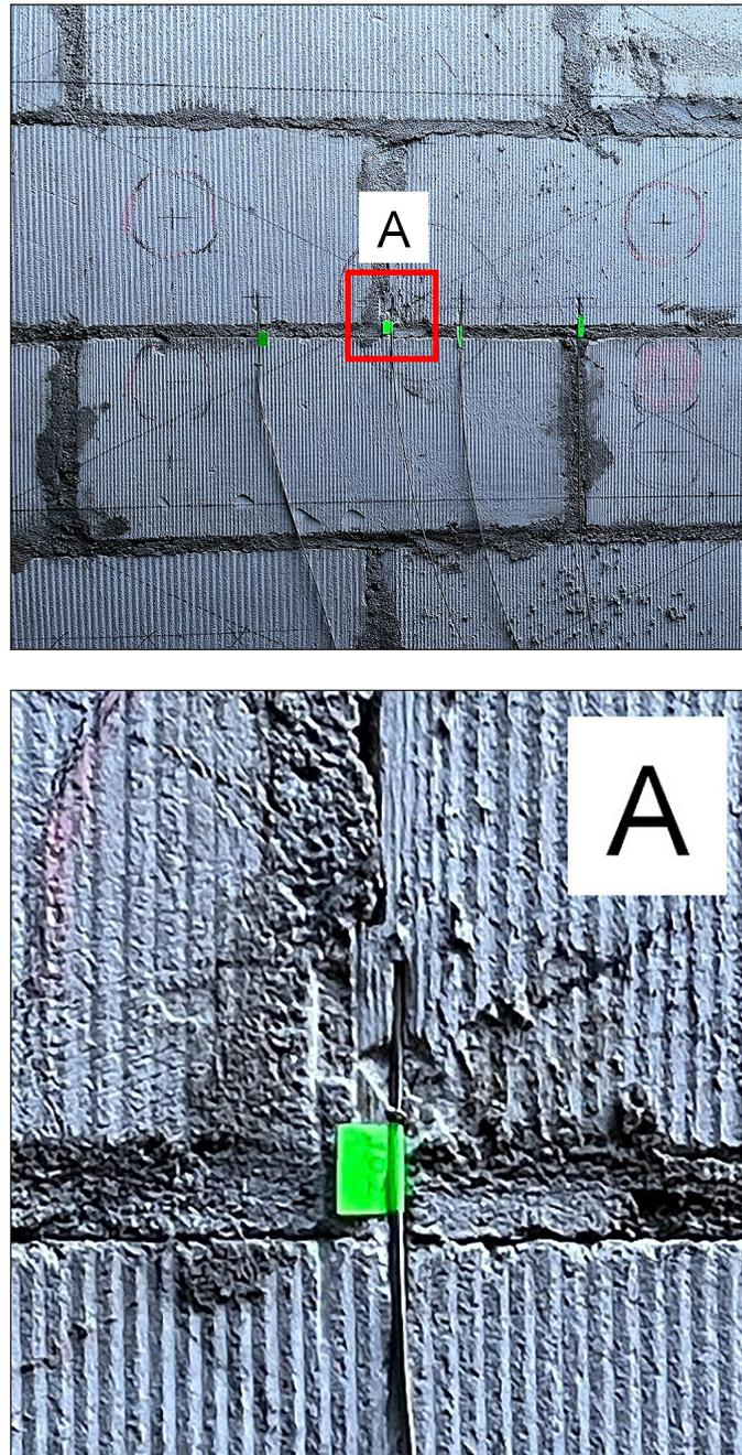
**Figure 10.** Thermocouples from measurement channels Ch101-Ch104 placed on the exterior side of the wall in the area not covered by the reflective-smoothing coating.
