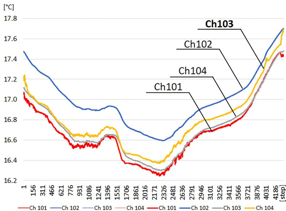
**Figure 9.** Measurement of the external wall temperature in the area not covered by the reflective-smoothing coating, during the representative 72-hour period
