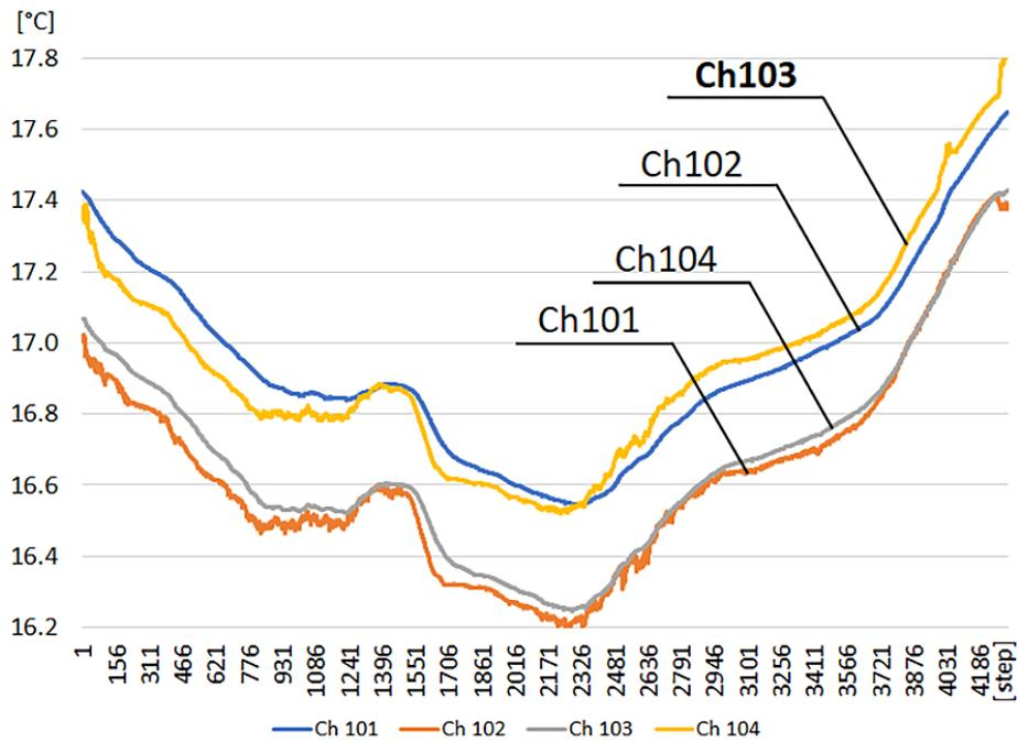
**Figure 11.** Measurement of the wall temperature in the area not covered by the reflective-smoothing coating, during the representative 72-hour period with values for channel Ch103 plotted after analysing the correlations between channels
