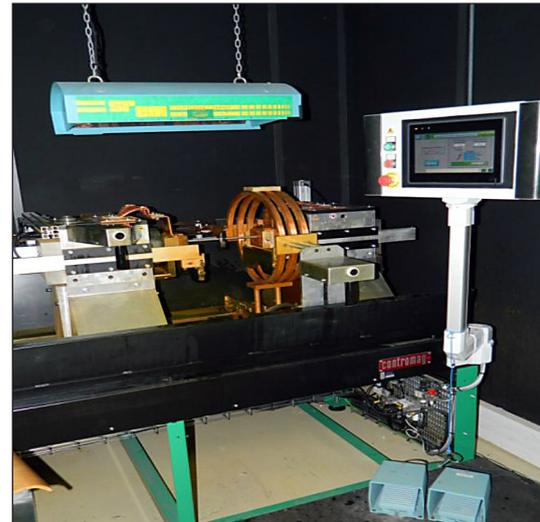
Fig. 7. CM 152 magnetic defectoscope
