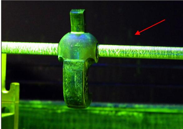
Fig. 8. Location of the defect in the test lock tongue
