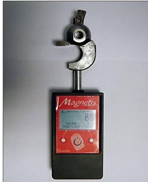
Fig. 9. The final measurement of residual magnetism in the tested component
