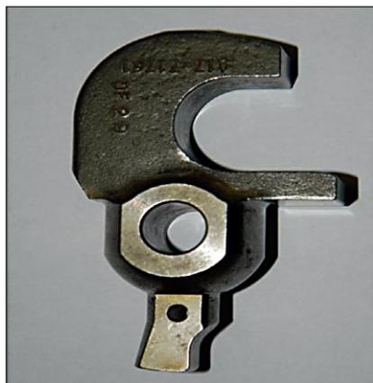
Fig. 1. The tested component – a lock tongue of a landing gear
