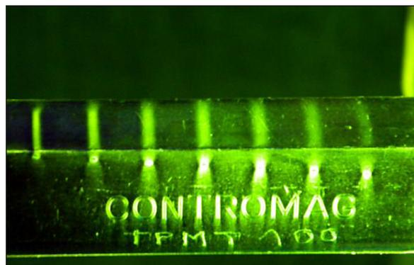
Fig. 4. The model Block A in UV lighting after completed magnetization and application of magnetic suspension
