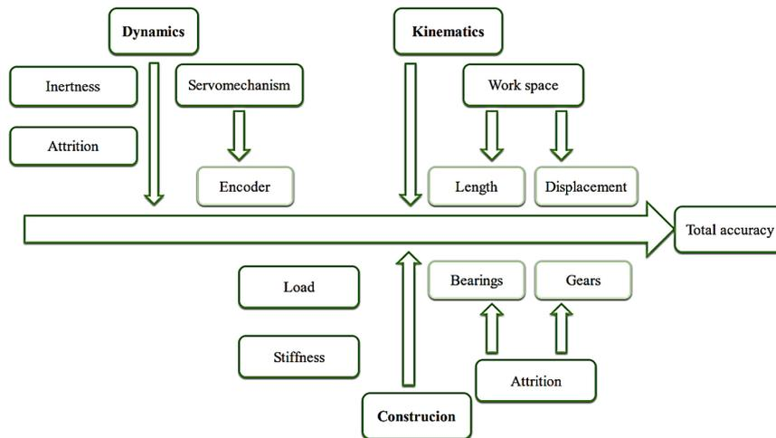
Figure 4. Sources of errors regarding the accuracy and repeatability of positioning of a milling plotter [14]
