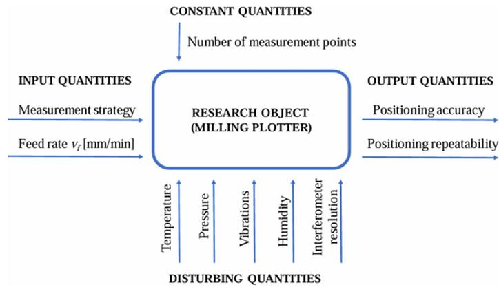
Figure 1. Research plan for assessing the accuracy and repeatability of positioning a three-axis CNC milling plotter
