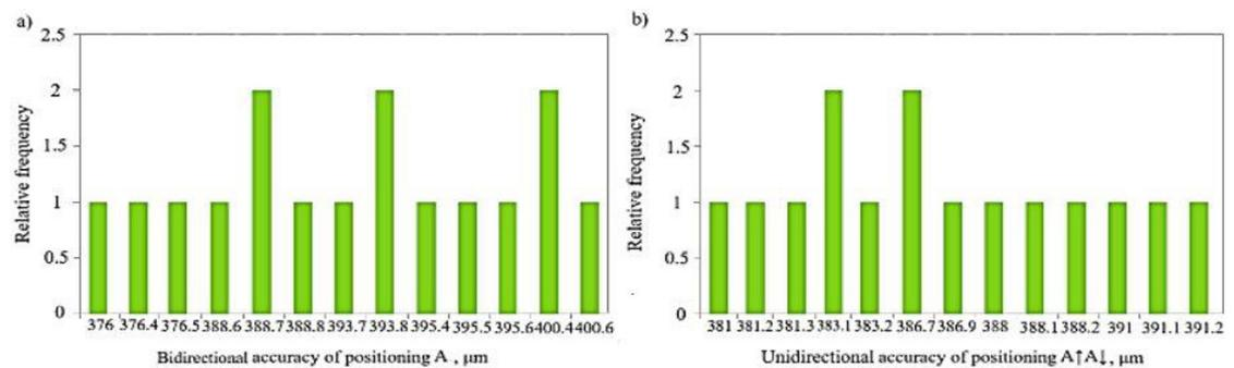
Figure 8. Frequency histograms of the milling plotter accuracy parameters values distribution obtained by the 'pilgrim' strategy: a) bidirectional accuracy of positioning, b) unidirectional accuracy of positioning
