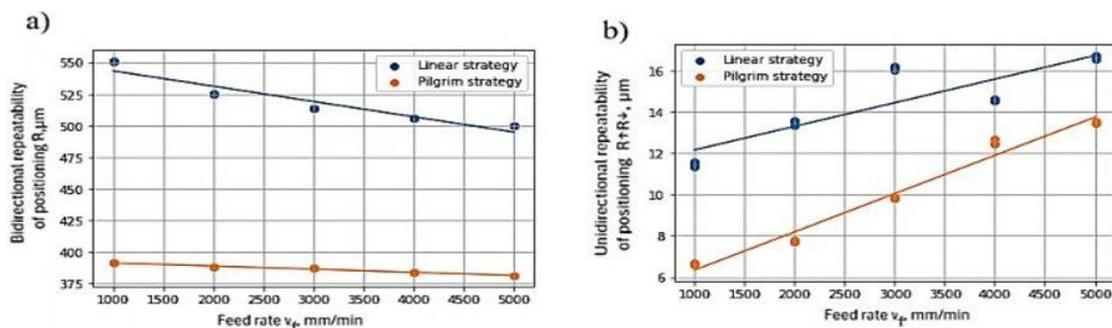
Figure 13. Positioning repeatability of the milling plotter: a) bidirectional repeatability, b) unidirectional repeatability
