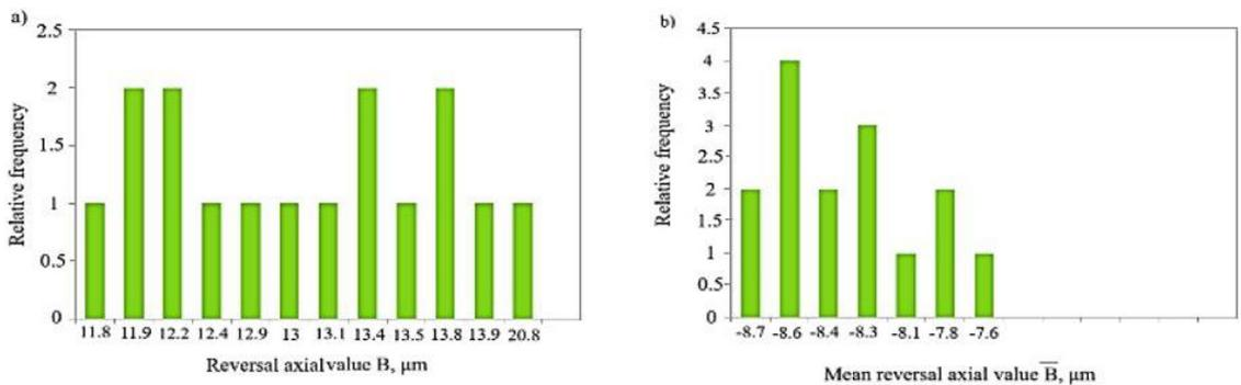
Figure 7. Frequency histograms of the milling plotter accuracy parameters values distribution obtained by the linear strategy: a) reversal axial value, b) mean reversal axial value
