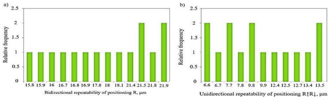
**Figure 9.** Frequency histograms of the milling plotter accuracy parameters values distribution obtained by the 'pilgrim' strategy: a) bidirectional repeatability of positioning, b) unidirectional repeatability of positioning
