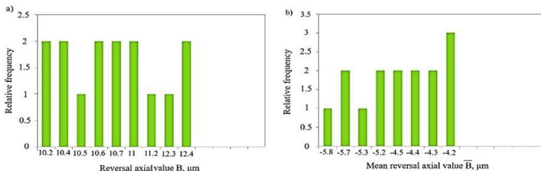
**Figure 10.** Frequency histograms of the milling plotter accuracy parameters values distribution obtained by the 'pilgrim' strategy: a) reversal axial value, b) mean reversal axial value
