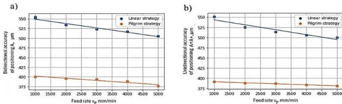
Figure 12. Positioning accuracy of the milling plotter: a) bidirectional accuracy, b) unidirectional accuracy
