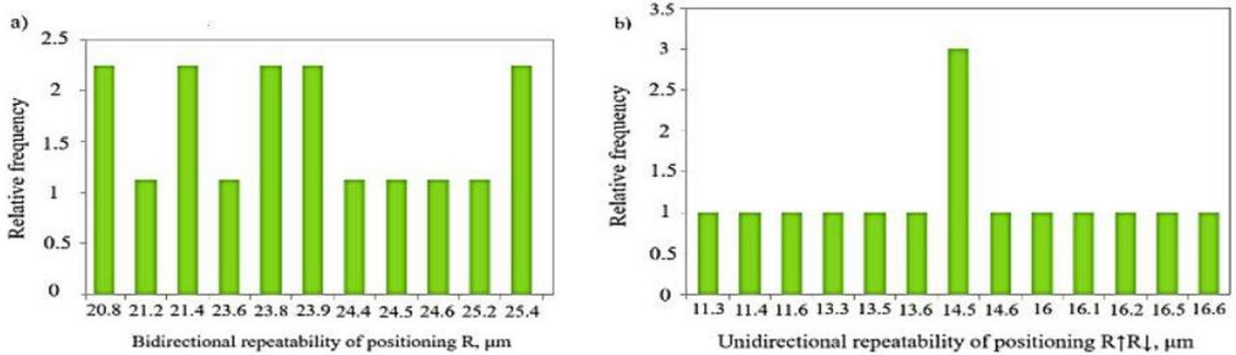
Figure 6. Frequency histograms of the milling plotter accuracy parameters values distribution obtained by the linear strategy: a) bidirectional repeatability of positioning, b) unidirectional repeatability of positioning
