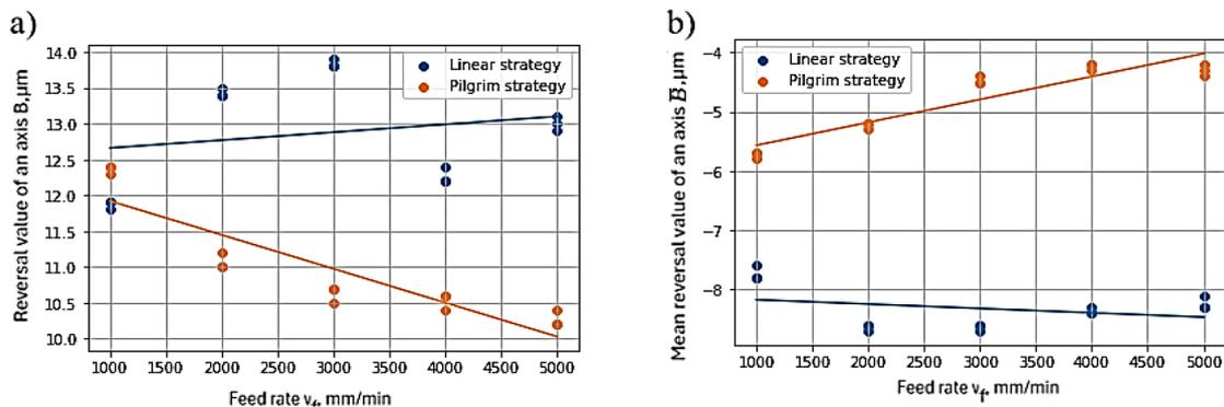
Figure 14. Reversal value of the milling plotter axis: a) reversal value, b) mean reversal value
