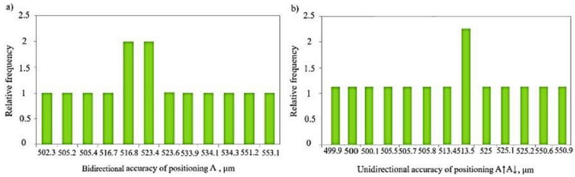
Figure 5. Frequency histograms of the milling plotter accuracy parameters values distribution obtained by the linear strategy: a) bidirectional accuracy of positioning, b) unidirectional accuracy of positioning
