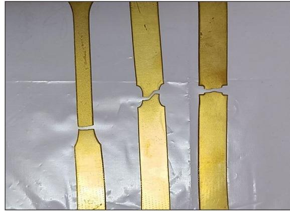
**Figure 8.** Tensile specimens after performing the tensile test
