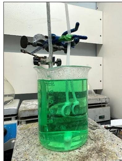
**Figure 1.** Ni-P electroless bath
