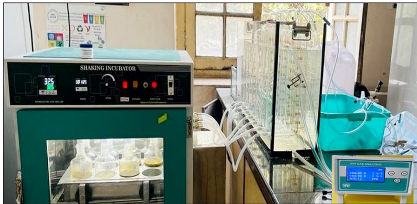
Figure 3. Photograph of experimental setup for biogas generation through anaerobic digestion
