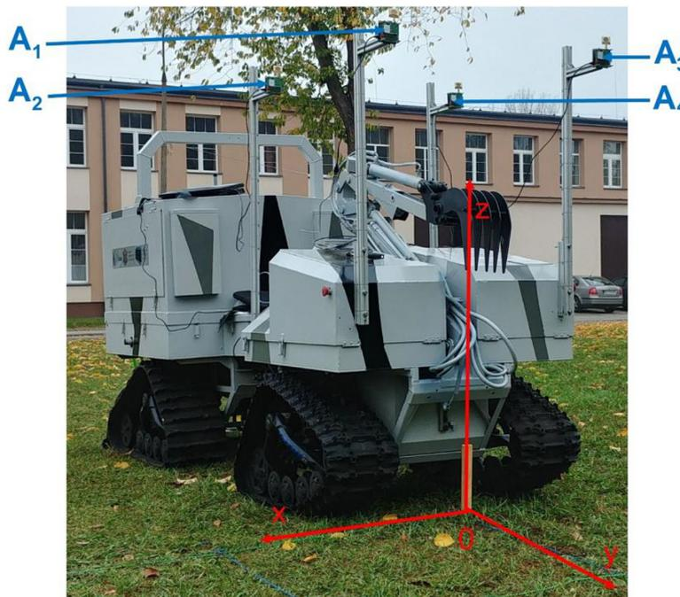
Figure 7. Anchor configuration on the UGV. Own elaboration based on [10]
