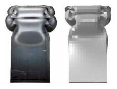
Fig. 4 Comparison of the final deformation mode between experimental and numerical models
