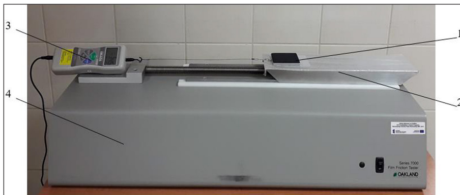
Figure 2. View of the frictional contact testing station: 1 – table with counter sample, 2 – track with measured sample, 3 – dynamometer, 4 – body
