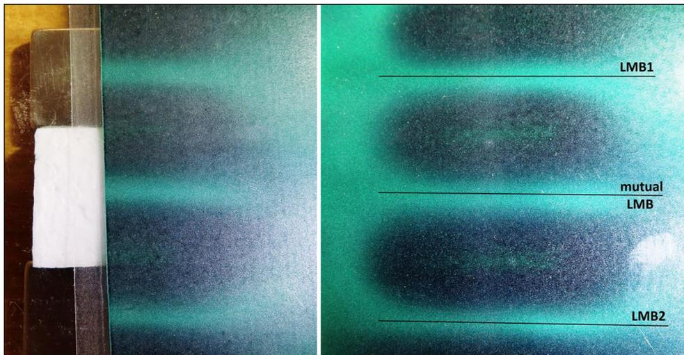
**Figure 9.** Two attracting permanent magnets separated by a piece of Styrofoam with their own interpoler lines (*LMB1*, *LMB2*) and one mutual line visible
