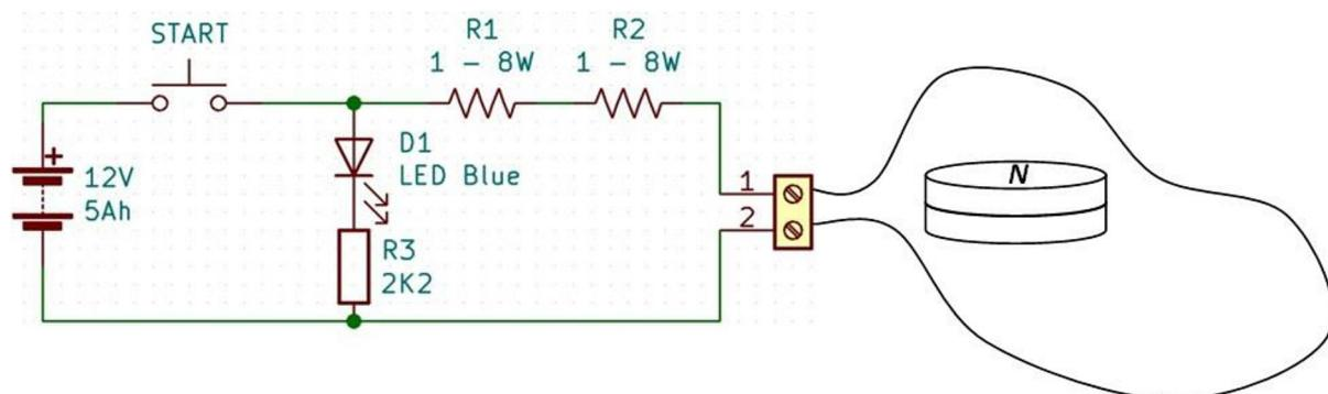
Figure 10. Electronic circuit diagram of experiment
