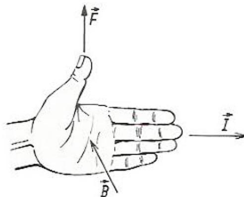
**Figure 3.** Mutual arrangement of the vectors: magnetic induction *B*, current *I* and force *F* according to Fleming's left-hand rule [15]
