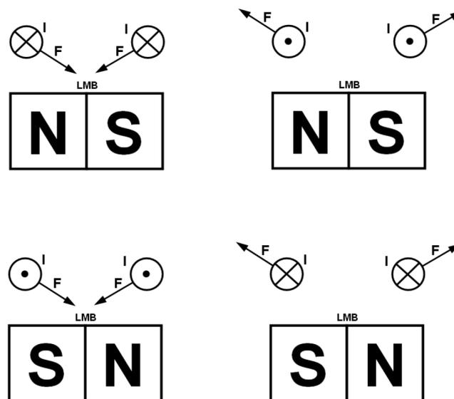
**Figure 13.** Four cases of force  $F$  acting on a conductor with current  $I$  near the *LMB* of a permanent magnet
