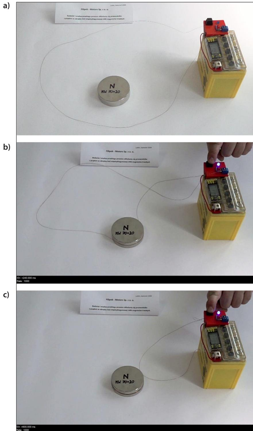
**Figure 11.** Experiment – initial state (a), experiment – 0.24 s after power on (b), experiment – 0.60 s after power on – termination (c)
