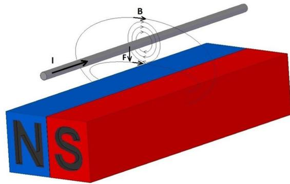
Figure 4. Interaction of magnetic field lines of a permanent magnet and a conductor with current
