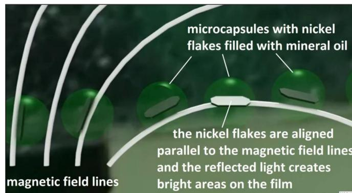
Figure 5. The principle of magnetic film [16]
