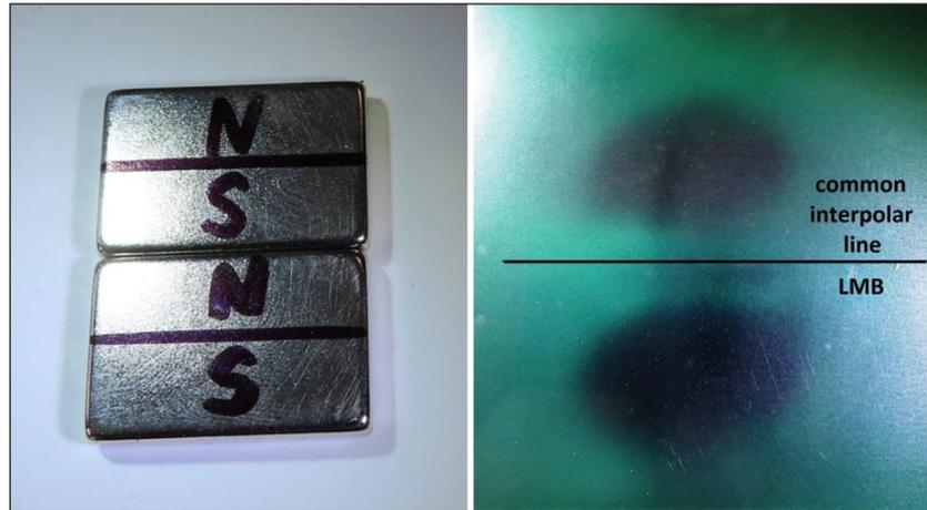
**Figure 8.** A mutual *LMB* line at the junction of two equal, connected permanent magnets observed with magnetic film
