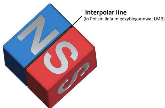
Figure 6. Representation of the location of the *LMB* line on the surface of a permanent magnet
