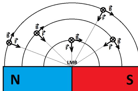
**Figure 2.** Schematic representation of the directions of the *F* force vectors acting on conductors with current
