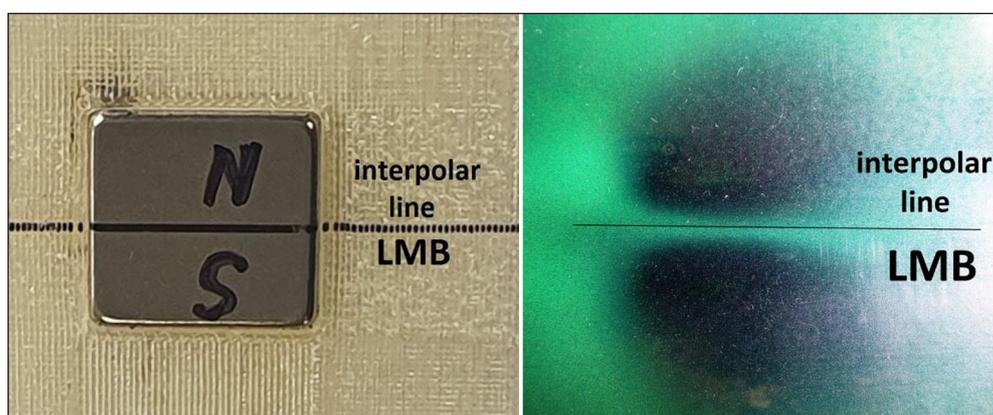
Figure 7. *LMB* line marked on the surface of an MPL 15x15x15/N38 permanent magnet and observed with magnetic film
