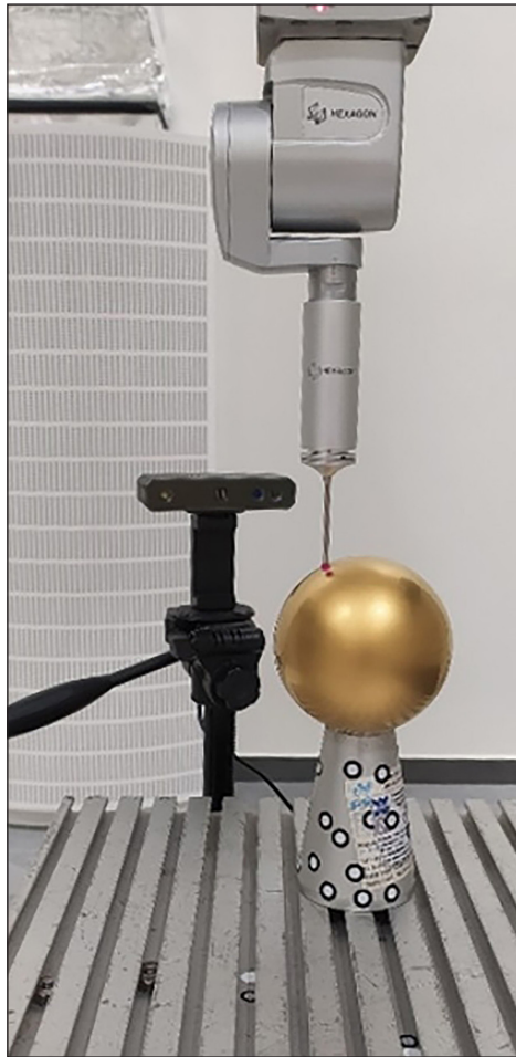
Figure 5. Measurements of reference sphere during tests on combined accuracy of hybrid measuring system (HMS) probing systems
