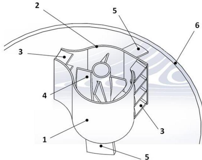
**Figure 2.** Screw impeller in a diffuser: 1, 2 – diffuser side surfaces, 3 – stream deflectors, 4 –screw impeller, 5 – supports, 6 – tank wall
