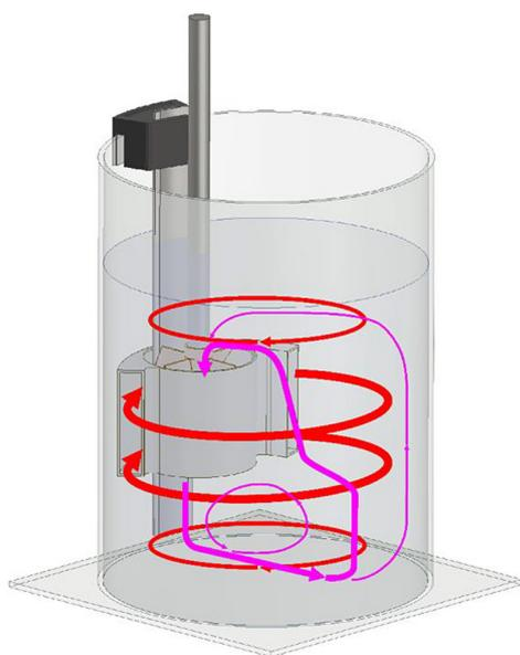
**Figure 3.** Liquid flow for an eccentric screw impeller in a side-flow diffuser
