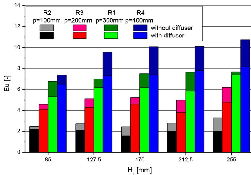
Figure 11. Power numbers of the tested impellers for turbulent mixing
