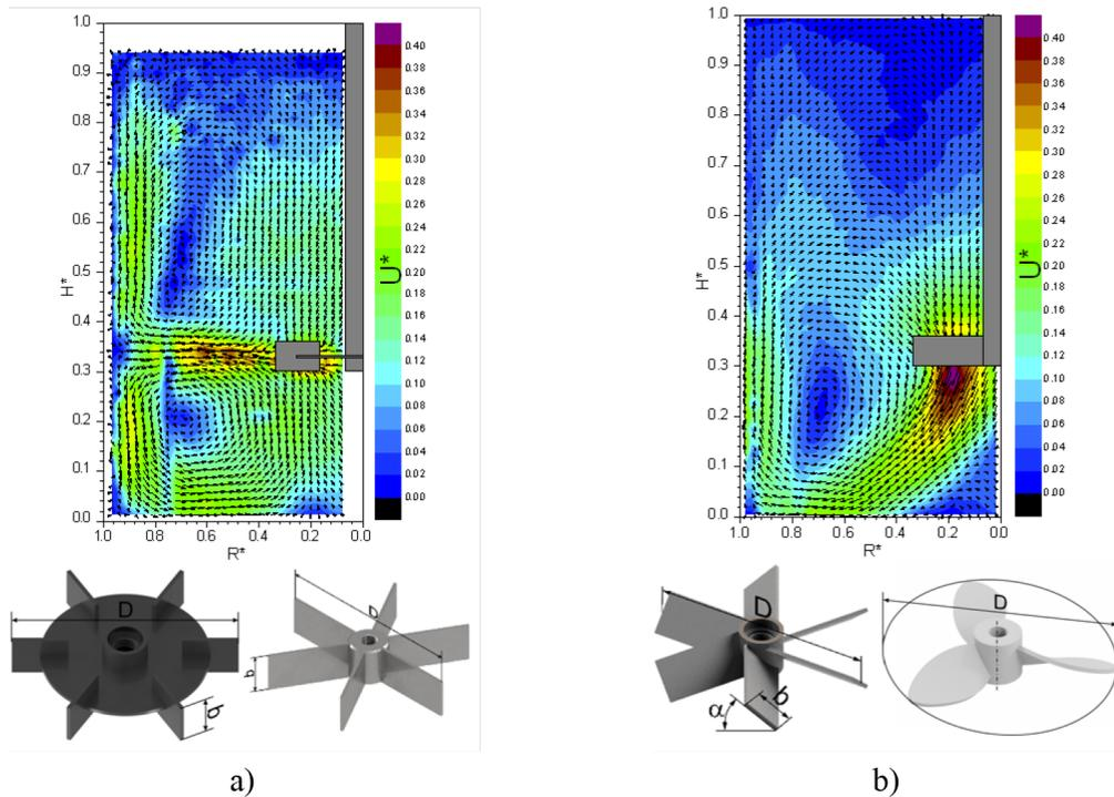
**Figure 1.** Methods of liquid circulation in a mixer and the impellers that generate them: (a) radial-circumferential, (b) axial-circumferential
