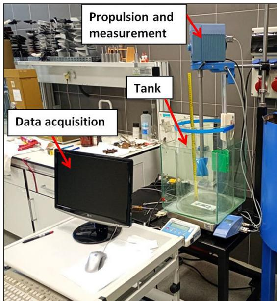
Figure 4. Photo of the test stand
