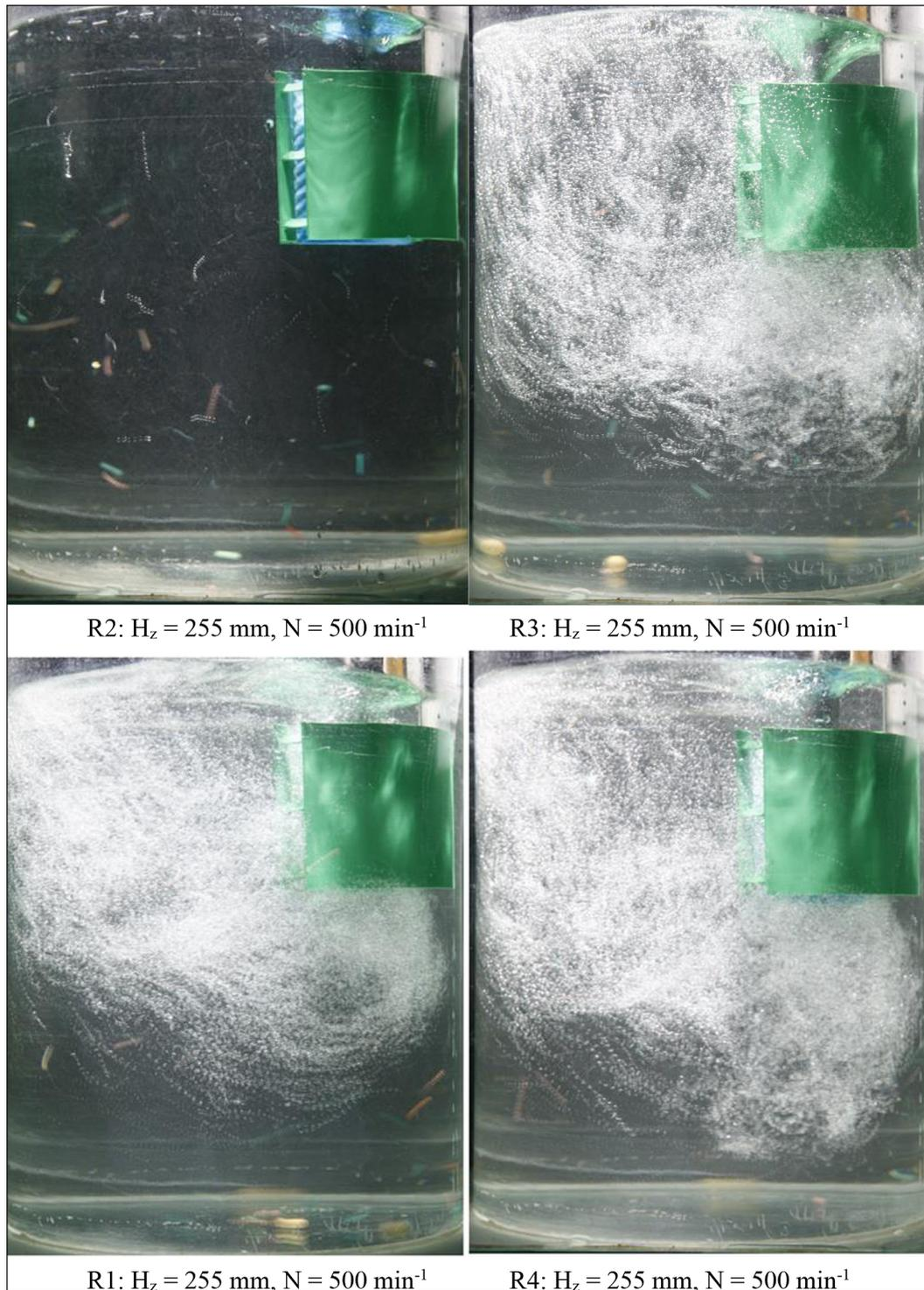
**Figure 6.** Trajectories of flow followers for high impeller placement
