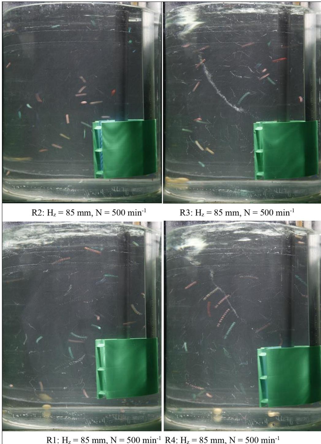
**Figure 7.** Trajectories of flow followers for low impeller placement
