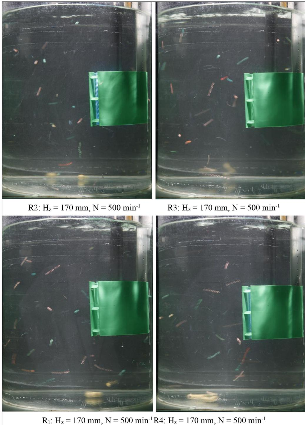
**Figure 8.** Trajectories of flow followers for central impeller placement
