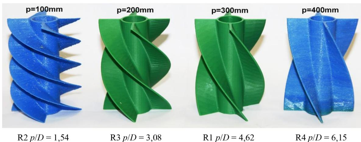
Figure 5. Investigated mixer impellers with different blade pitches
