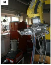
Figure 1. Cold spray: (a) schematic [9], (b) Impact Innovations 5/8 high-pressure system
