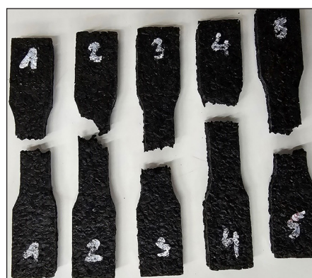
Figure 9. View of samples after tensile test
