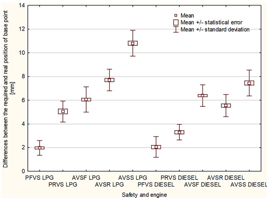
Figure 5. A comparison of changes in floor panel geometry in cars after covering a mileage of 300,000 km, depending on the vehicle safety type and the fuel supply system type
