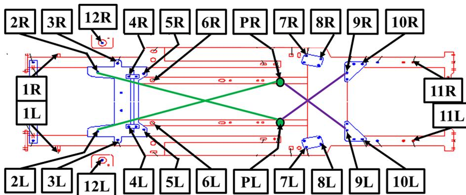
Figure 2. The distribution of points at which the geometry of the floor panel and the McPherson struts was measured
