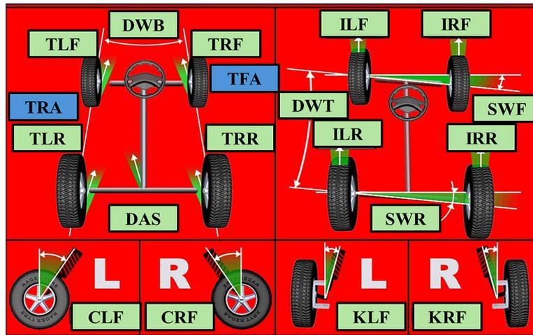
Figure 3. The wheel alignment parameters identified during testing
