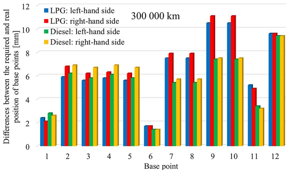
Figure 4. Changes in geometry of the floor panel and the upper mounting of the McPherson struts after a mileage of 300,000 km in cars with compression-ignition (Diesel) engines and with LPG-fuelled engines
