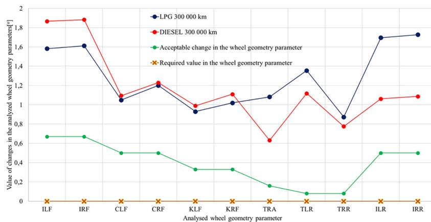
**Figure 6.** Changes in wheel alignment in the cars with compression ignition (diesel) engines and with LPG-fuelled engines
