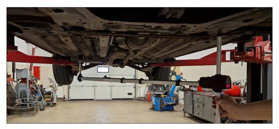
Figure 1. A view of the floor panel and a body geometry measuring instrument
