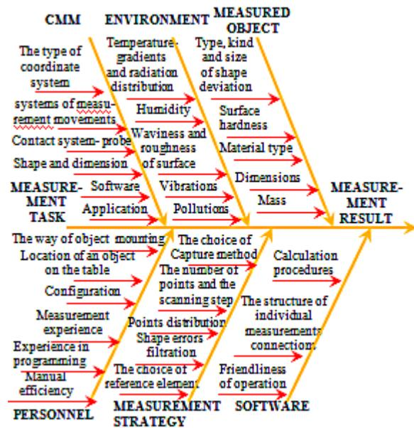
Fig. 6. Ishikawa diagram developed for the process of assessment of measurement error [15]
