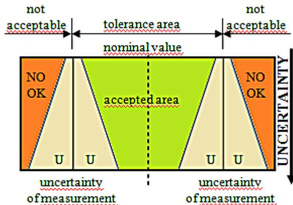
Fig. 5. Measurement uncertainty: the range of uncertainty reduces the fields of compliance and non-compliance [15]
