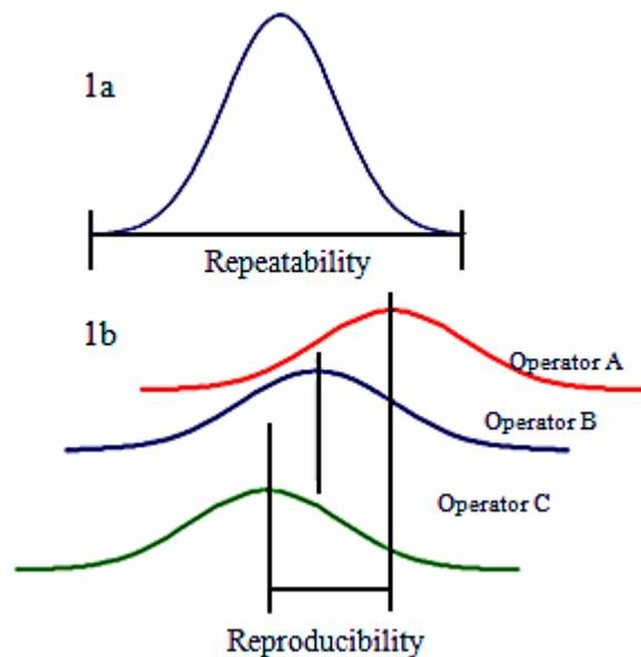
Fig. 1. Graphical interpretation of a) repeatability b) reproducibility of measurements
