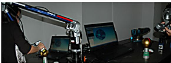
Fig. 4. Measuring CPA with optical probe [6]
