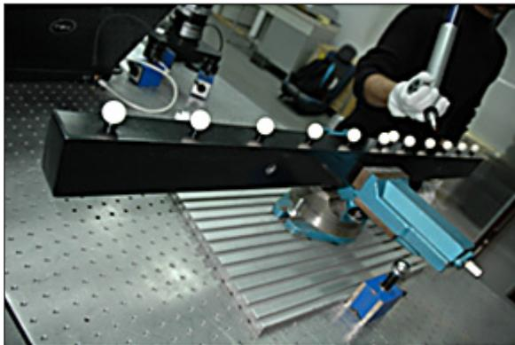
Fig. 3. Measuring station with Ball-Bar artefact
