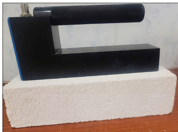
Figure 3. TDR narrow surface sensor on a cellular concrete sample
