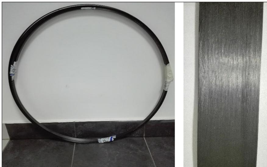
Figure 1. CFRP tape from S&P Polska
