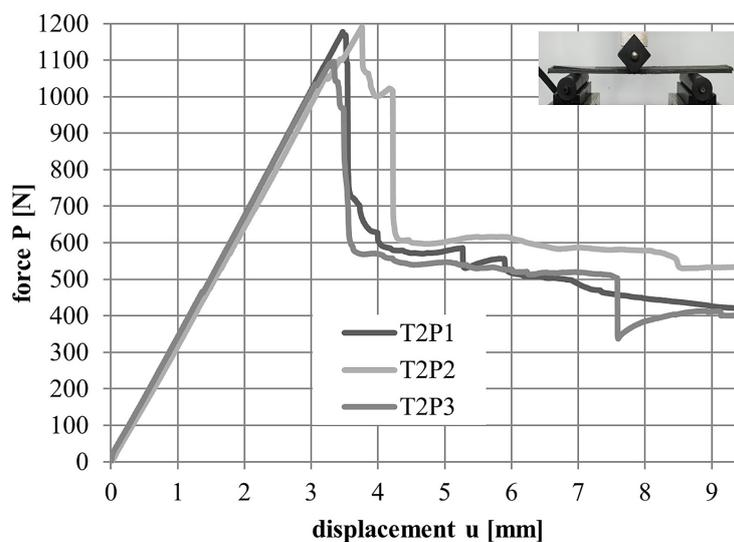
Figure 6. The relationship of force P as a function of displacement u for the T2 series
