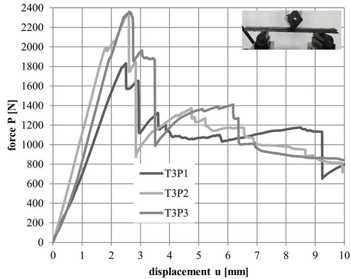
Figure 7. The relationship of force  $P$  as a function of displacement  $u$  for the T3 series
