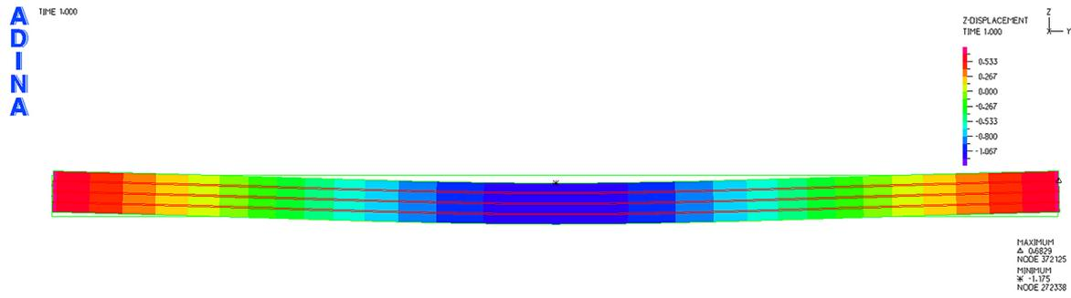
Figure 18. Displacement of the T4P strips with a load of 3423.76 N
