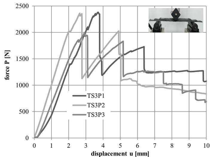
**Figure 10.** The relationship of force P as a function of displacement u for the TS3 series
