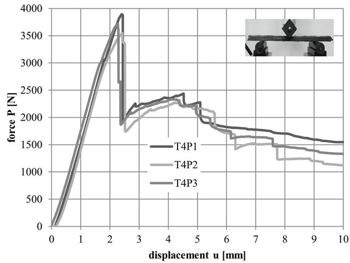
Figure 8. The relationship of force  $P$  as a function of displacement  $u$  for the T4 series
