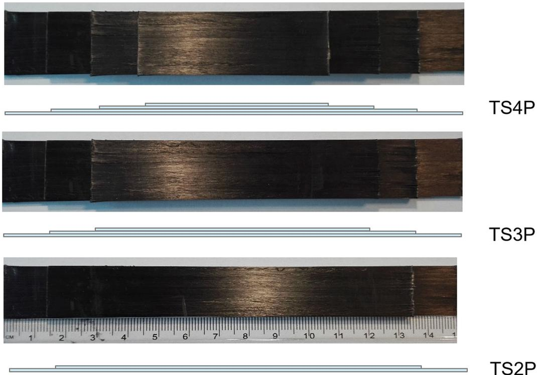
**Figure 4.** Scheme and designation of progressive samples, where: T– CFRP strip, S – sample with shortened CFRP strip, number (L) – denotes the number of strips
