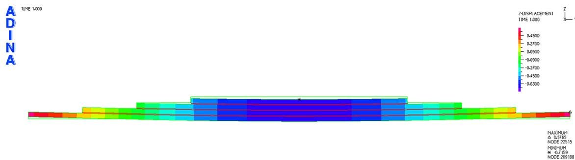
Figure 21. Displacement of the TS4P strips with a load of 1691.91 N
