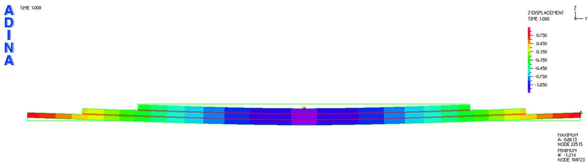
Figure 20. Displacement of the TS3P strips with a load of 1612.98 N
