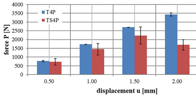
Figure 14. Comparison of P force values in T4P and TS4P strips for assumed displacement values u = 0.5; 1; 1.5 and 2 mm
