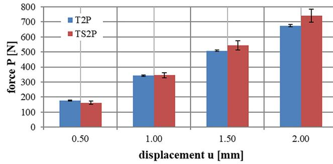
Figure 12. Comparison of P force values in T2P and TS2P for assumed displacement values u = 0.5; 1; 1.5 and 2 mm
