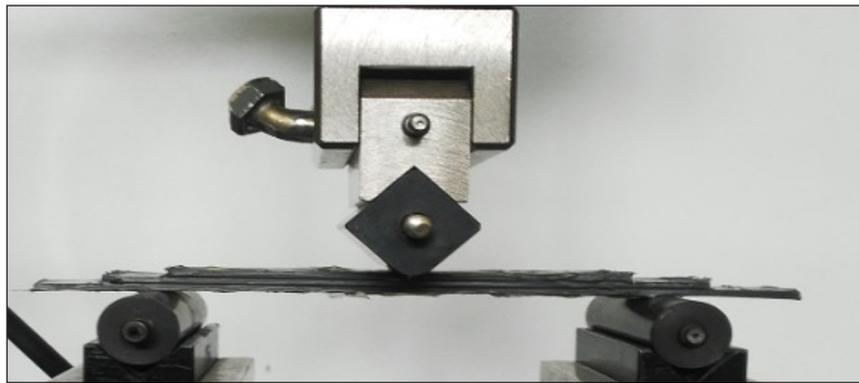
Figure 5. Sample mounted in the three-point bending holder
