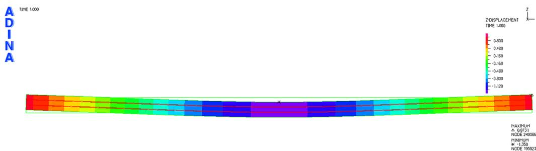
Figure 17. Displacement of the T3P strips with a load of 1830.44 N
