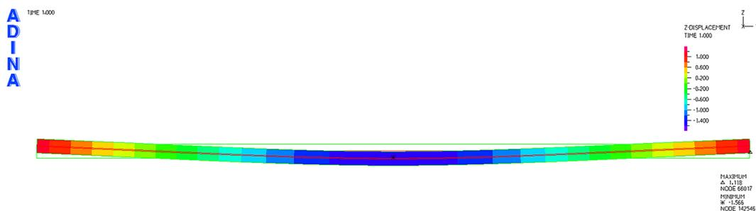
Figure 16. Displacement of the T2P strips with a load of 674.33 N
