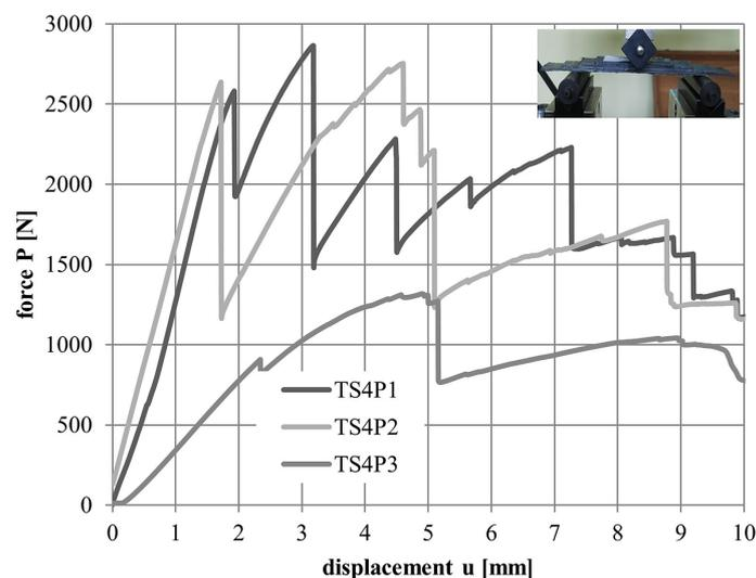
**Figure 11.** The relationship of force P as a function of displacement u for the TS4 series
