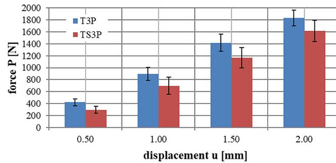
Figure 13. Comparison of P force values in T3P and TS3P strips for assumed displacement values u = 0.5; 1; 1.5 and 2 mm
