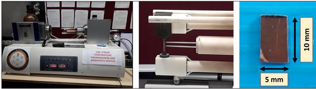
Figure 4. (a) Schematic of LINSEIS standard LSR-3 measurement system and (b) LSR-3 System probes connected to the specimen. (c) Test Specimens and their dimensions for testing conductivity on LSR-3
