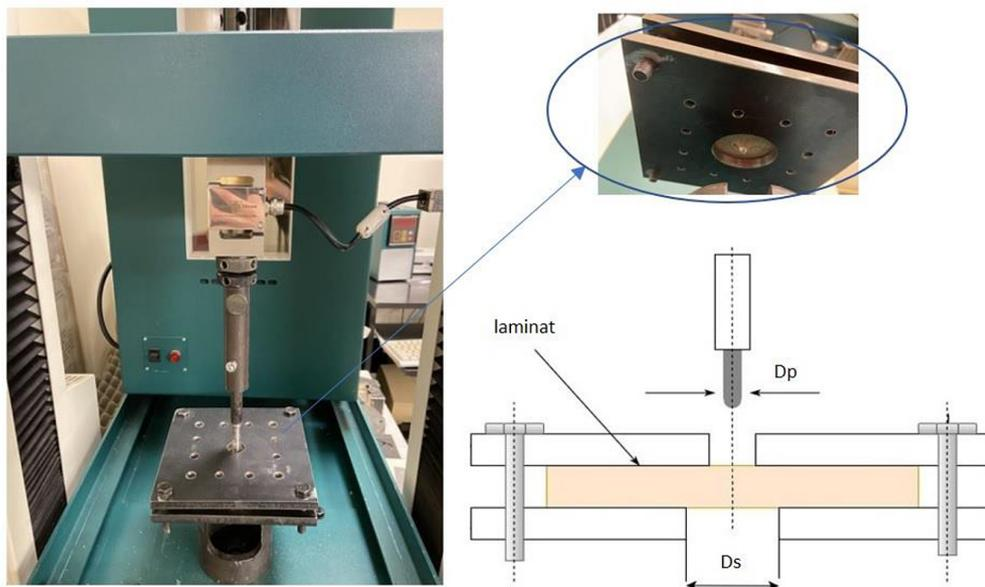
**Figure 3.** Schematic of the quasi-static punch shear test fixture. D<sub>p</sub> – punch diameter, D<sub>s</sub> – support diameter
