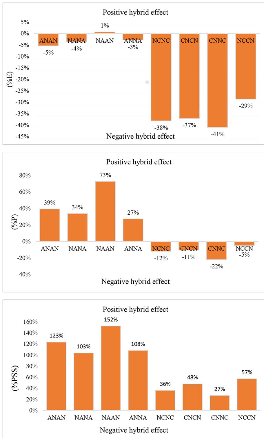
**Figure 10.** The effect of hybridization compared to natural laminates (calculations based on averaged values)
