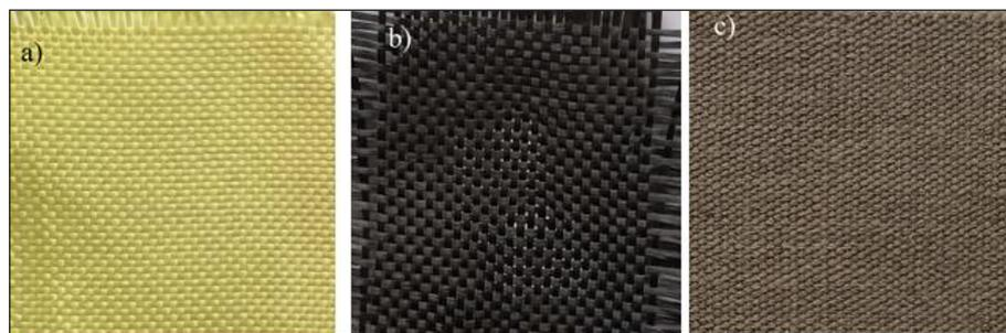
Figure 1. Fabrics used as reinforcement of laminates: a) aramid, b) carbon, c) natural (flax)
