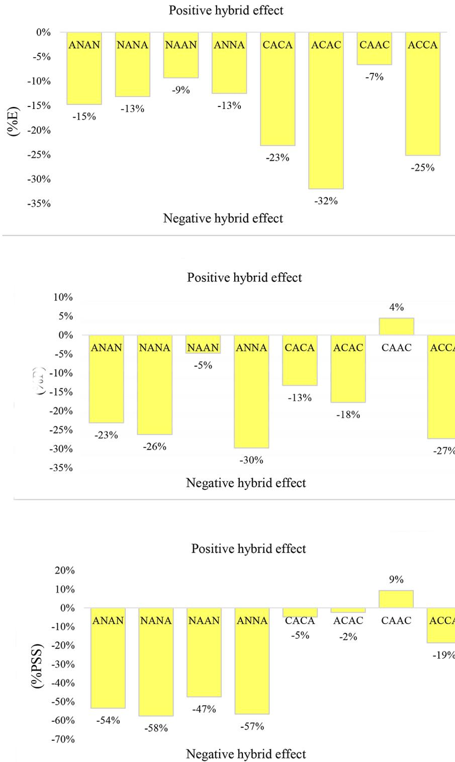
**Figure 9.** The effect of hybridization compared to aramid laminates, (calculations based on averaged values)
