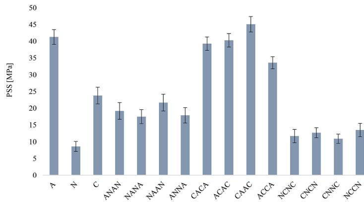
Figure 6. PSS comparison of hybrid and non-hybrid laminates
