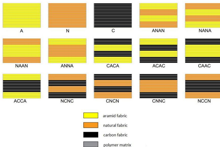
Figure 2. Reinforcement layer configuration in laminates
