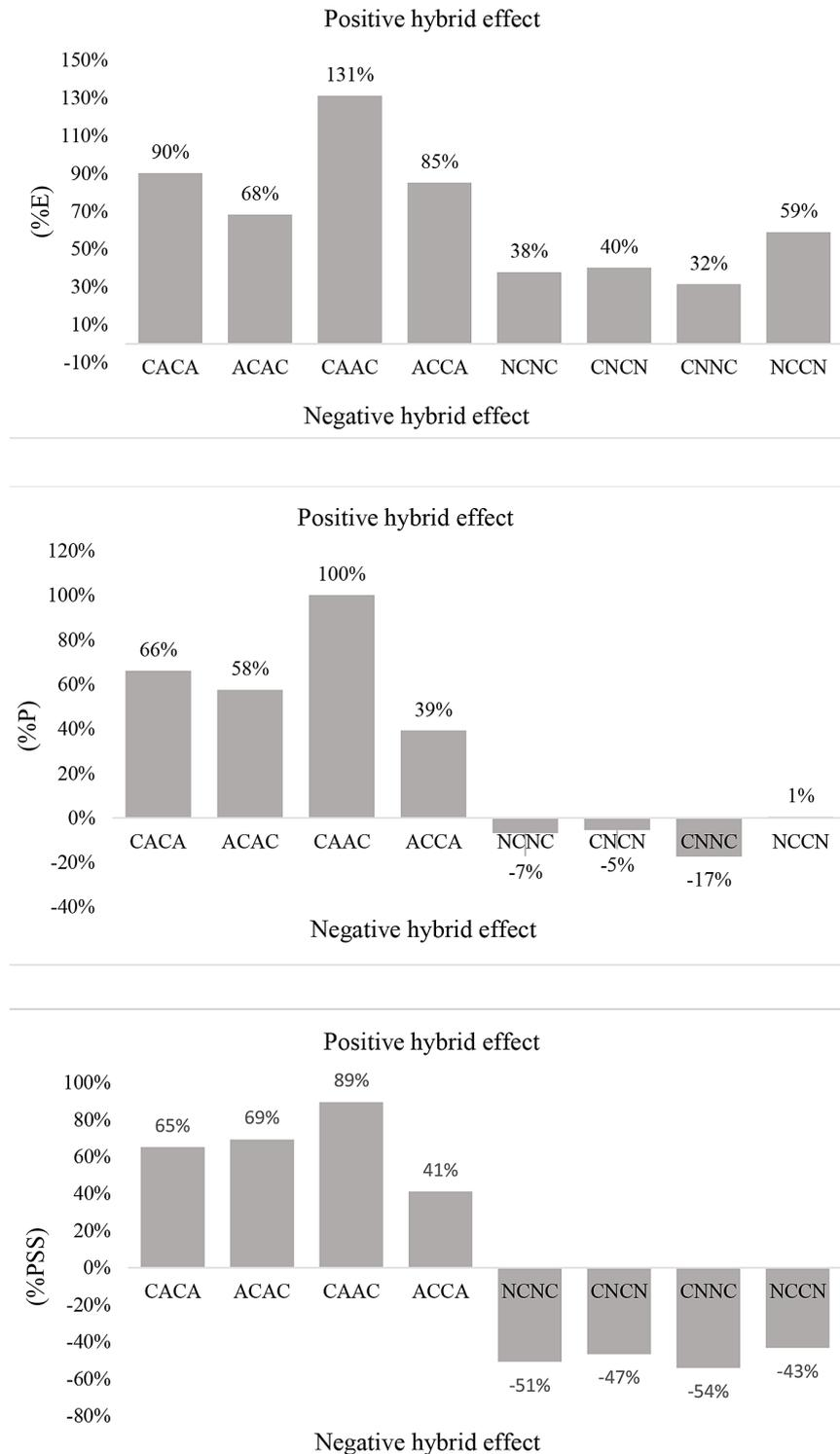
**Figure 11.** The effect of hybridization compared to carbon laminates (calculations based on averaged values)
