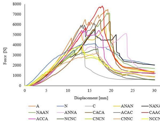
**Figure 5.** Penetration force-displacement curves of hybrid and non-hybrid laminates
