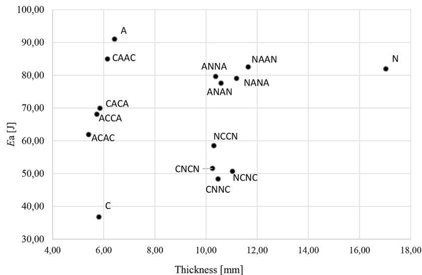
Figure 8. Effect of laminate thickness on energy absorption
