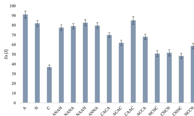
Figure 7. Comparison of absorbed energy (Ea) values for hybrid and non-hybrid laminates
