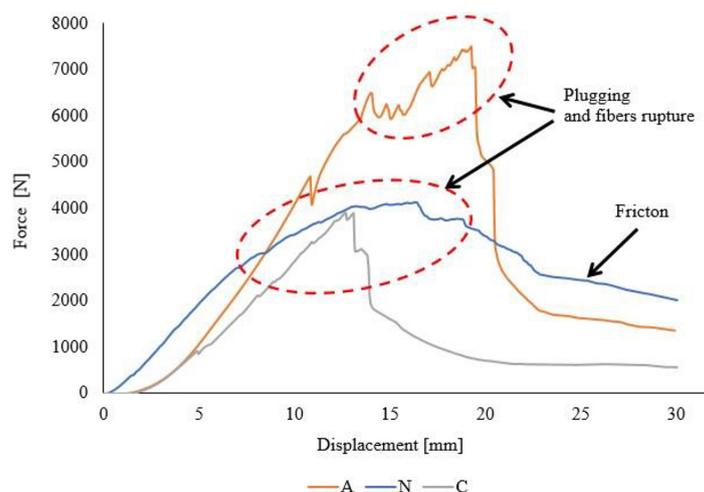
Figure 4. Force as a function of displacement for non-hybrid laminates
