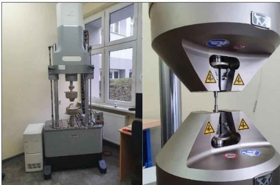
Figure 2. Instron ElectroPuls E1000 test stand
