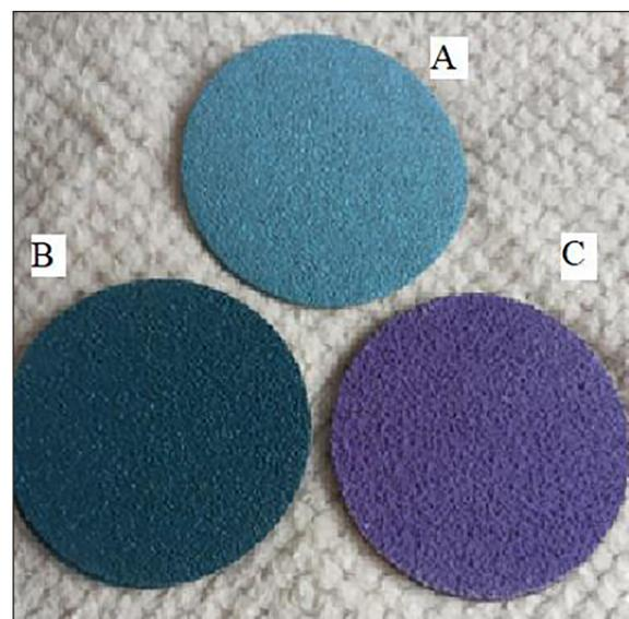
**Figure 1.** Grinding discs with abrasive grains: A) electrocorundum; B) zirconium; C) ceramic
