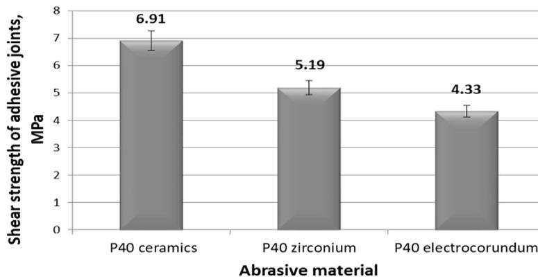
**Figure 8.** Shear strength of adhesive joints whose adherends surfaces have been ground using three abrasive materials: ceramics, zirconium, electrocorundum
