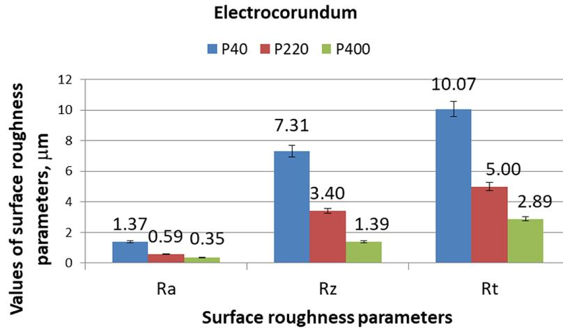
**Figure 5.** Surface roughness parameters of adherends after treatment with electrocorundum with gradations: P40, P220, P400
