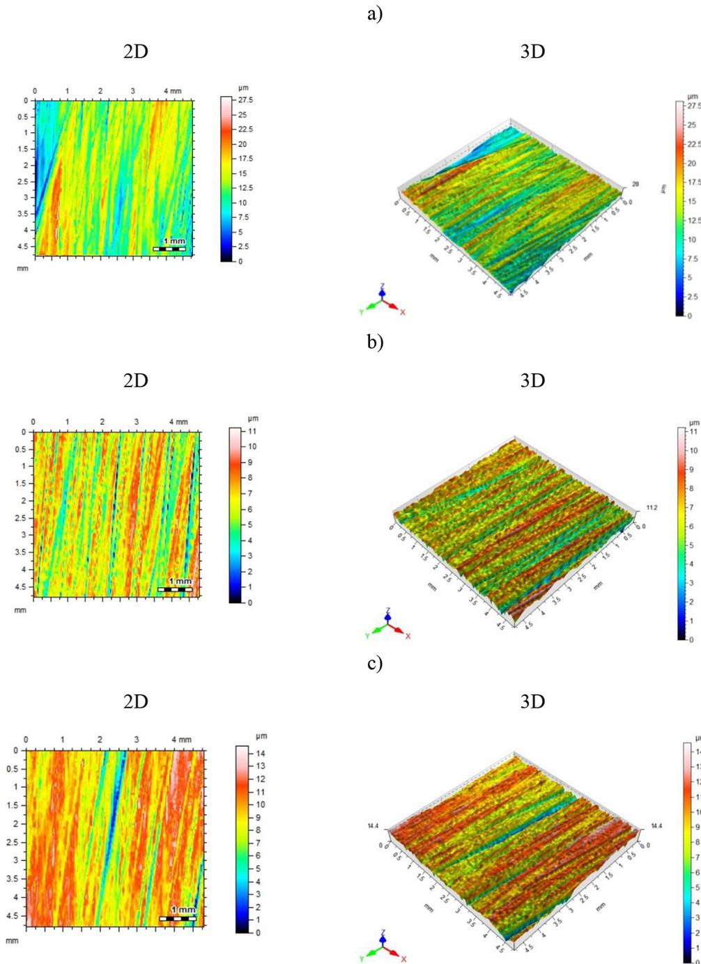
**Figure 6.** 2D and 3D surface roughness maps for adherends surfaces prepared with various types of abrasive grains: a) P40 ceramics, b) P40 zirconium, c) P40 electrocorundum
