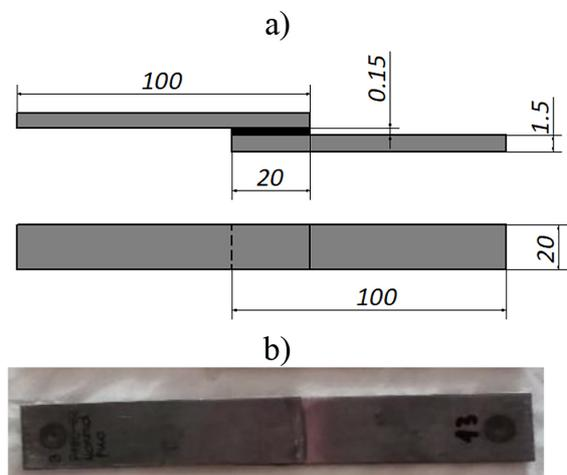
**Figure 3.** Adhesive joints sample: a) scheme, b) view
