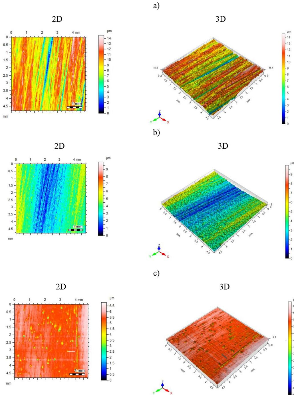
**Figure 7.** 2D surface roughness charts for adherends surfaces prepared with the same abrasive material (electrocorundum) with different gradations: a) P40 b) P220, c) P400
