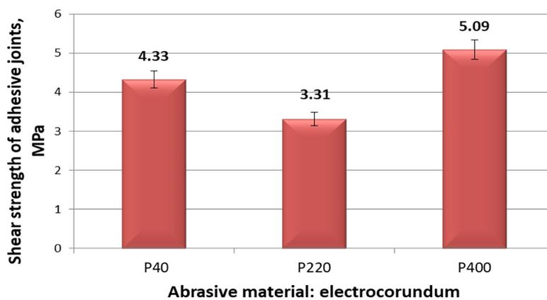
**Figure 9.** Shear strength of adhesive joints whose adherends surfaces have been ground using three grades of electrocorundum: P40, P220, P400
