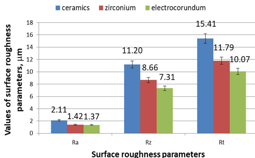
Figure 4. Summary of 2D surface roughness parameter results depending on the type of abrasive material
