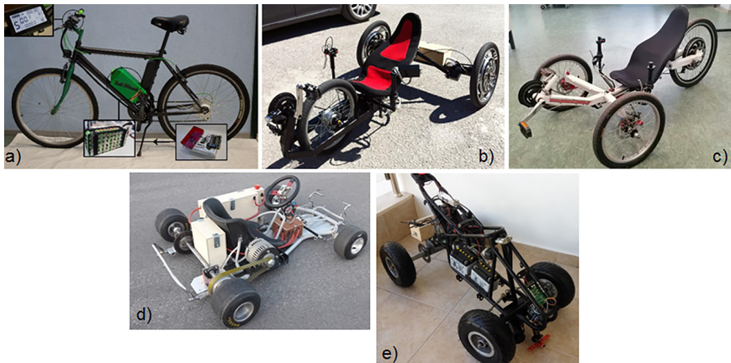
Figure 3. Small scale vehicles of the Laboratory of Energy Systems of the International Hellenic University used for the Student Transitional project: a) electric bicycle, b) delta type electric tri-cycle, c) tad-pole type electric tri-cycle, d) electric go-kart, e) small scale electric utility vehicle with the ability to perform semi-autonomous movement
