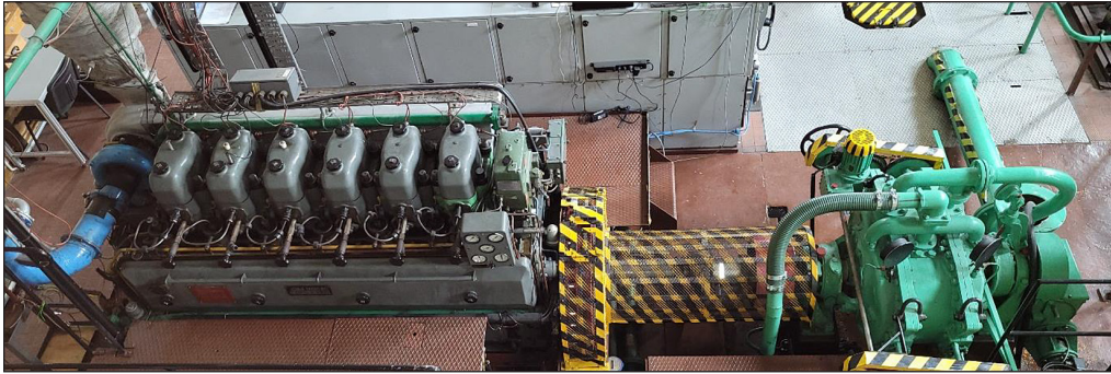
Figure 5. Test stand of Sulzer 6 AL 20/24 marine engine with a water brake on the right
