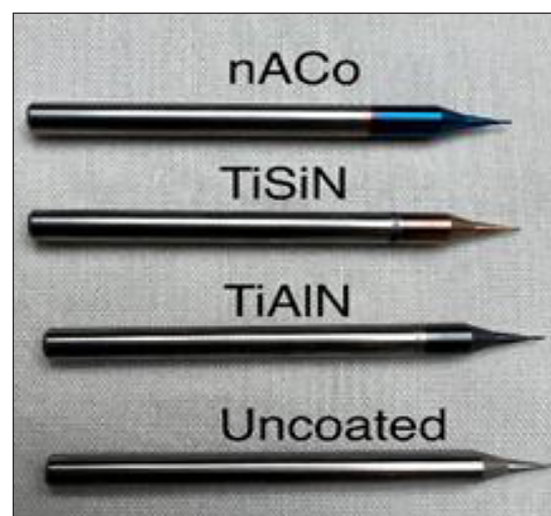
Figure 3. Multiple coated micro tools
