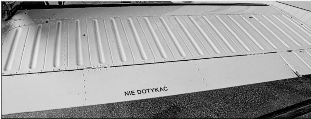
**Figure 1.** An example of the application of embossing in the aircraft tail covering
