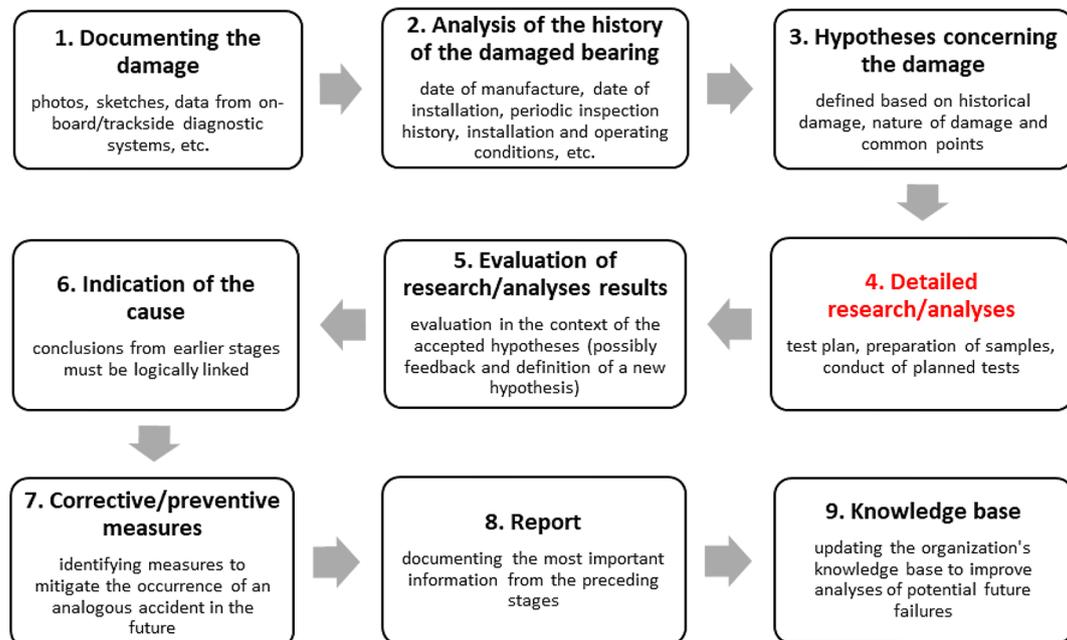
**Figure 2.** Block diagram of the research method for analyzing the cause of damage to wheelset bearings
