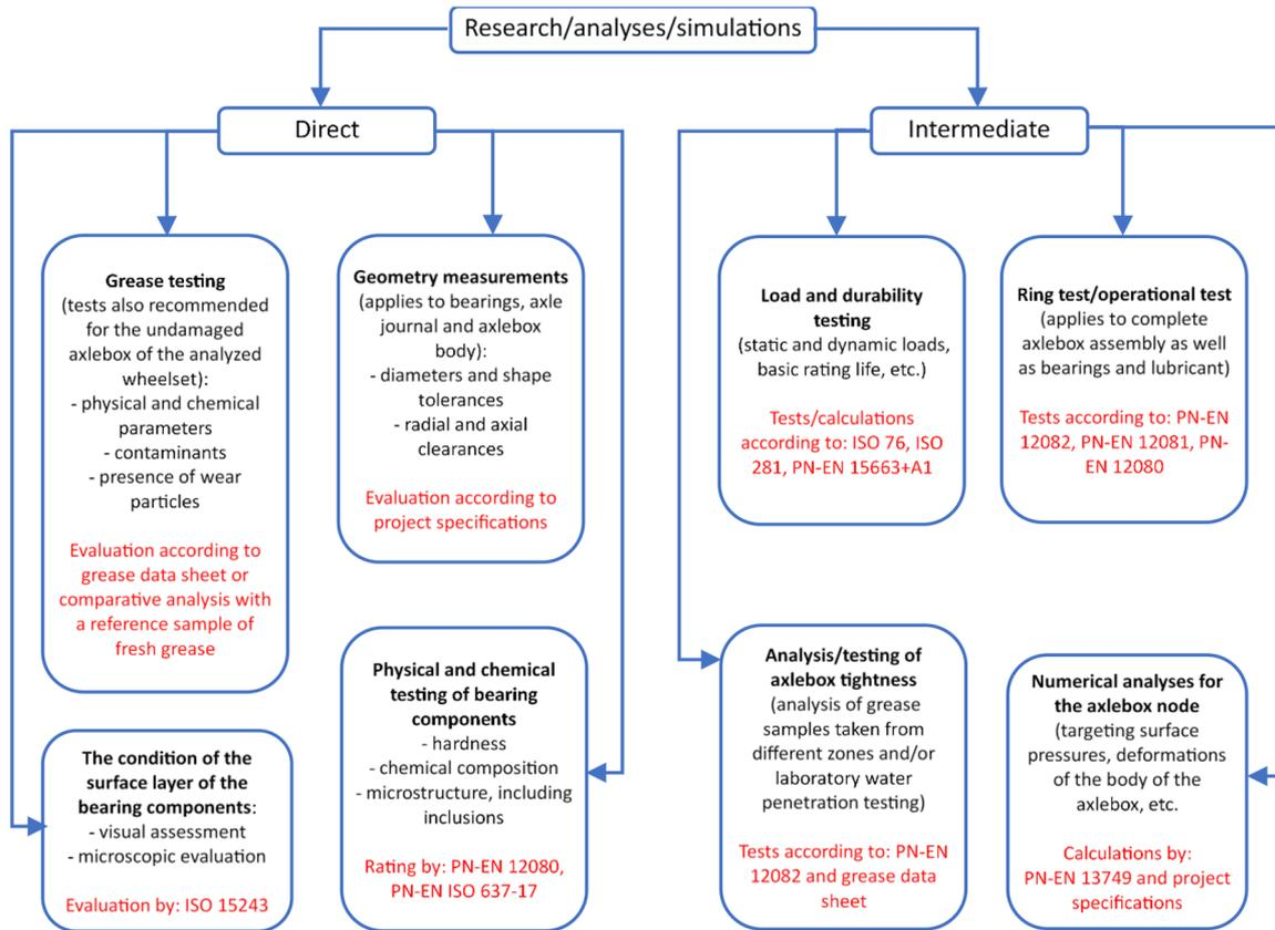
Figure 3. Expanded block diagram of the research method applied for step 4 from Figure 2
