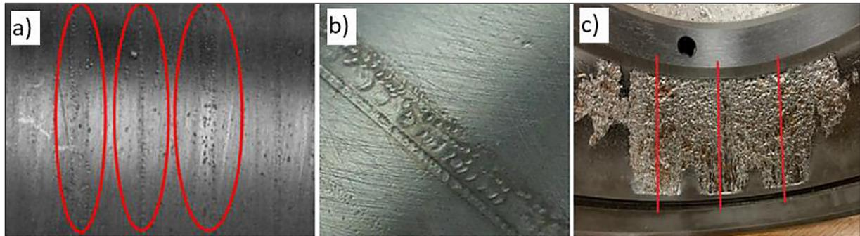
Figure 5. Photographs of sample damage: (a), (b) current leakage erosion, (c) moisture corrosion (photos: P. Biel)
