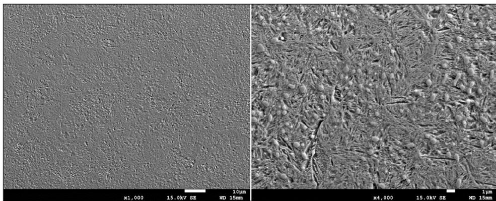
Figure 6. Microstructure of a sample taken from the outer race of an NJ bearing, 100 CrMo7 steel, from SKF Company – prepared by Institute of Ferrous Metallurgy in Research paper report no. N0-0912. Gliwice, 2021
