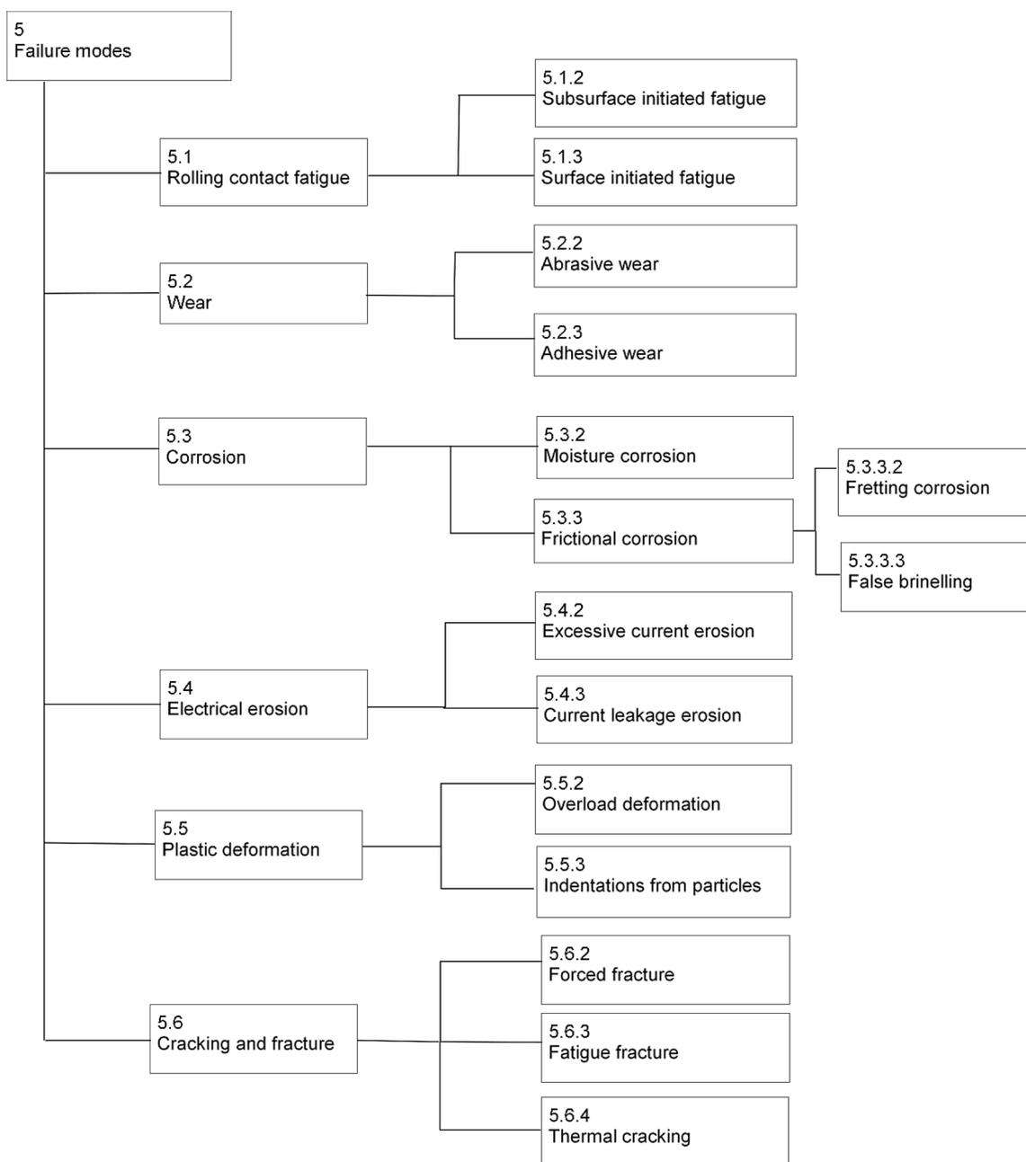
Figure 1. Classification of bearing failure mode [5]
