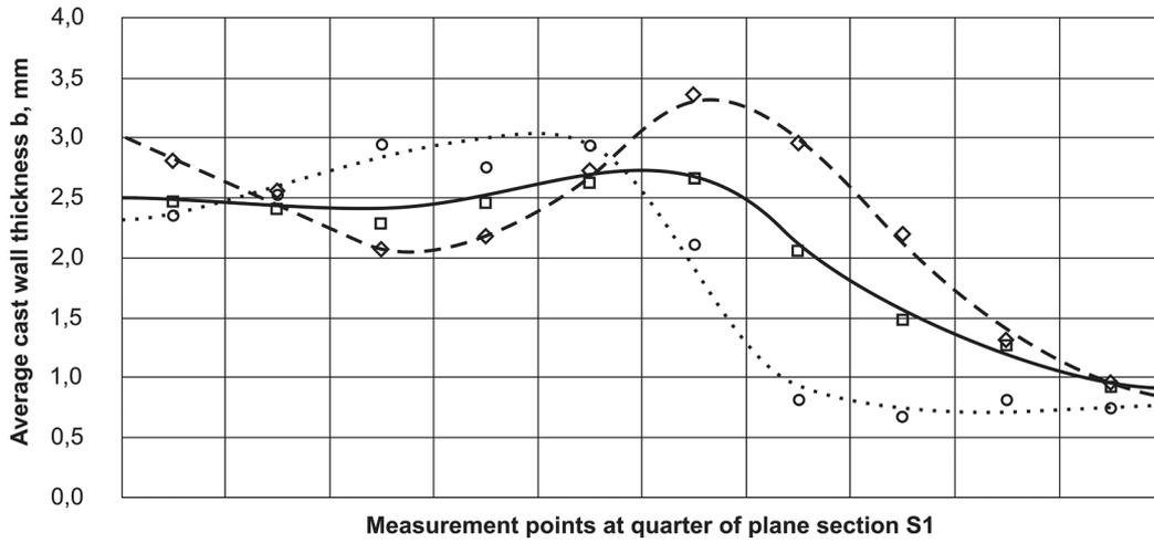
Fig. 5. Changes in average cast wall thickness  $b$  in plane section S1:  $R_{or} = 1$  (full line),  $R_{or} = 1.25$  (dashed line),  $R_{or} = 1.67$  (dotted line)
