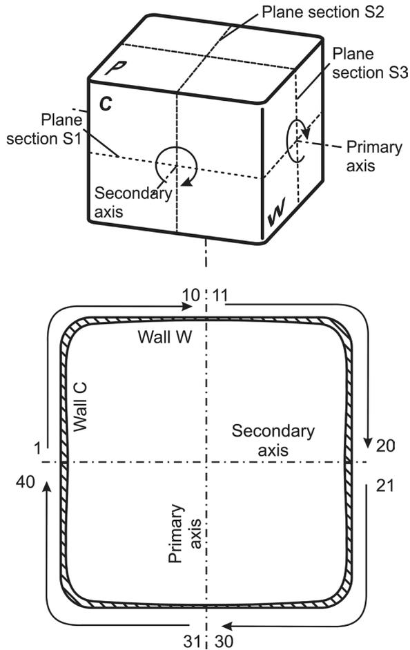
**Fig. 4.** a) positions of plane sections S1, S2 and S3 relative to main and auxiliary axes of rotation, b) example of position of measurement points at plane section S1
