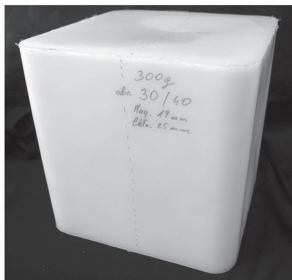
**Fig. 3.** Cast produced in rotational molding
