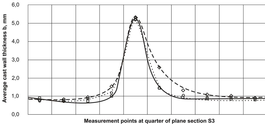
Fig. 7. Changes in average wall thickness  $b$  in plane section S3:  $R_{or} = 1$  (full line),  $R_{or} = 1.25$  (dashed line),  $R_{or} = 1.67$  (dotted line)
