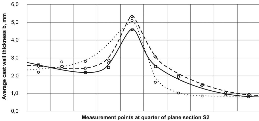
Fig. 6. Changes in average wall thickness  $b$  in plane section S2:  $R_{or} = 1$  (full line),  $R_{or} = 1.25$  (dashed line),  $R_{or} = 1.67$  (dotted line)
