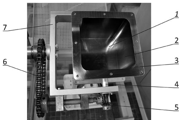
**Fig. 2.** Auxiliary axis rotation unit and mold for rotational molding: 1 – bottom head of mold, 2 – mold plate, 3 – collar for fastening upper head, 4 – journal bearing, 5 – bevel gear, 6 – chain transmission, 7 – arm
