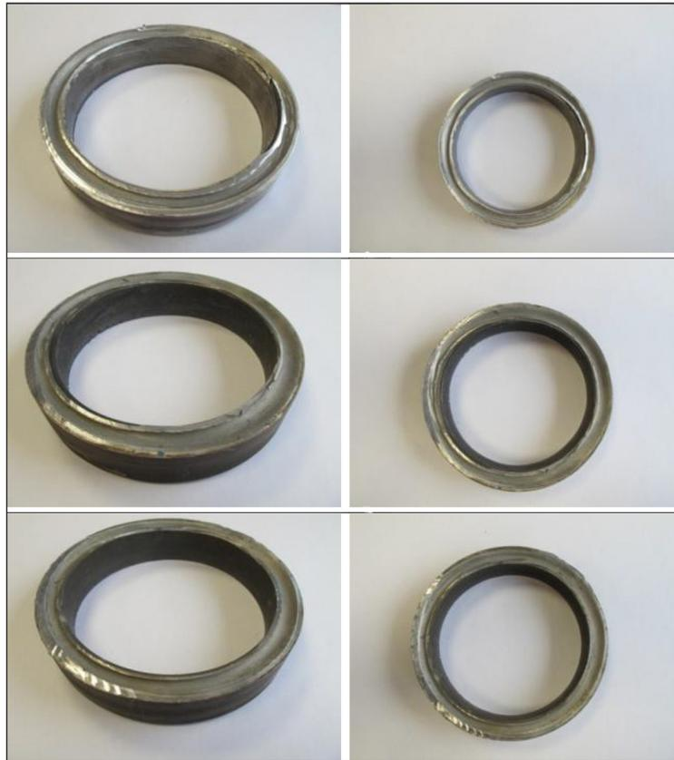
Figure 17. Example rings made on the experimental rolling mill
