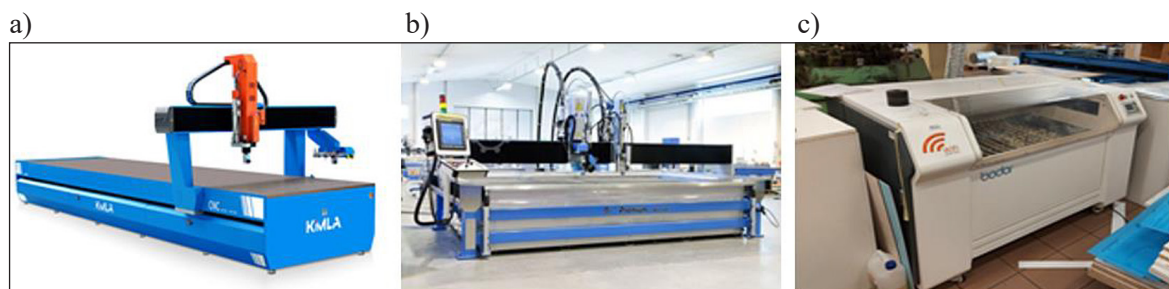
Figure 2. Tools used for composite cutting (a) plotter of a milling machine KIMLA BPF2160, (b) Water Jet Sweden NCP 4020D BEV (3D), (c) laser plotter BODOR BCL -1005X
