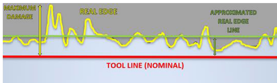
Figure 5. Research methodology scheme: magnified photography with characteristic lines, marked: * red – nominal line representing position of the cutting tool, * yellow line – real line representing edges after cutting * green – approximation of edges after cutting, reduced to a straight line
