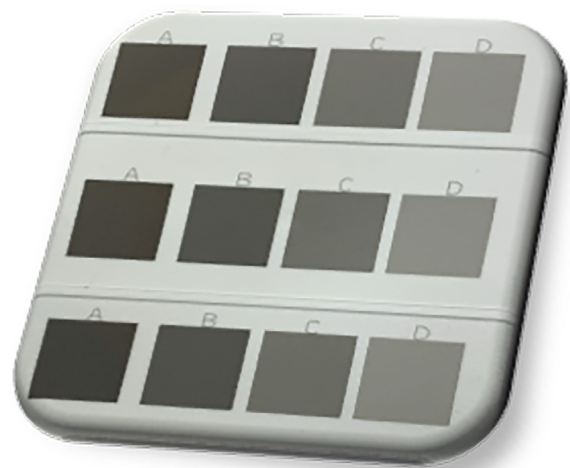
Figure 1. Test sample with laser marked signs with various parameters of laser beam
