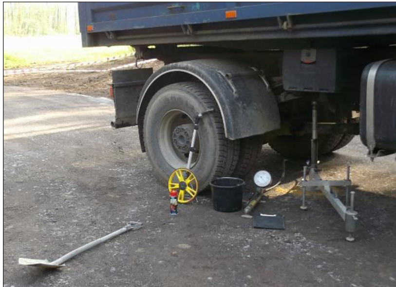
Figure 1. Static plate load test on a forest road – test device
