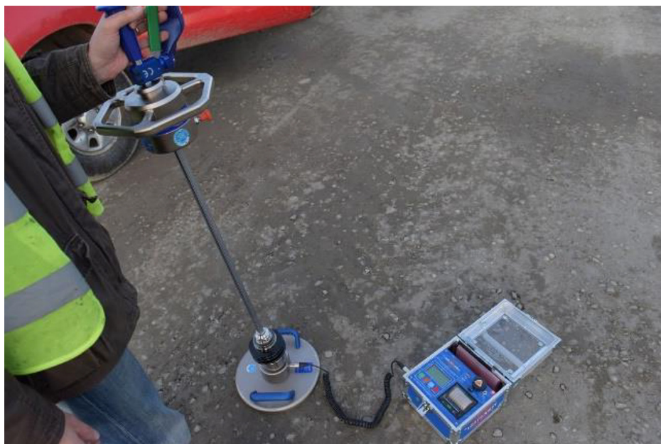
Figure 3. Dynamic plate load test on a forest road – test device
