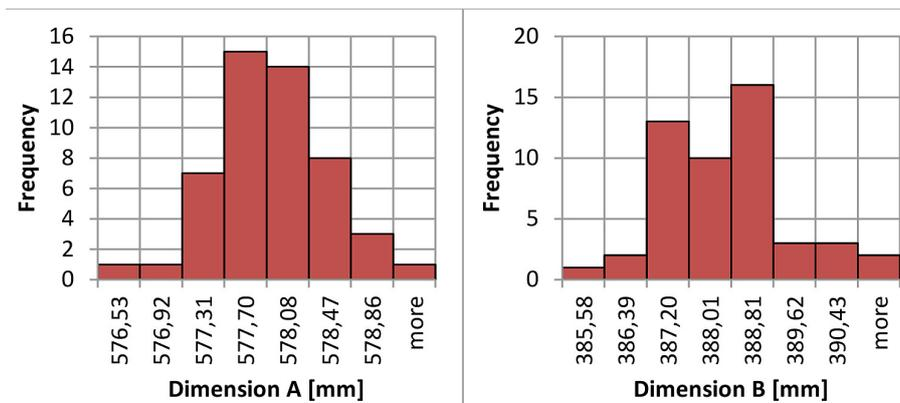
Figure 6. Histogram of dimension A [mm] (left side); dimension B [mm] (right side) – efficiency 20 pcs/min (cardboard packaging No. 1)
