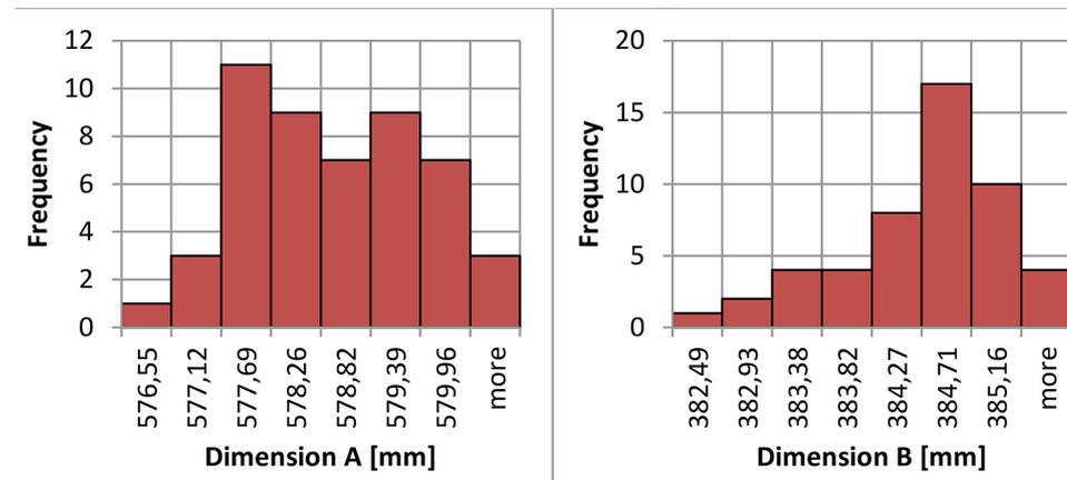
Figure 10. Histogram of dimension A [mm] (left side); dimension B [mm] (right side) – efficiency 15 pcs/min (cardboard packaging No. 1)
