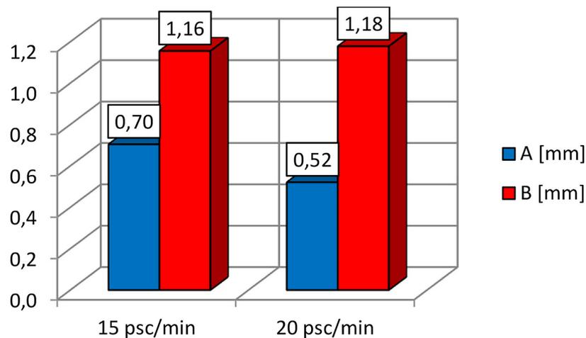
**Figure 8.** Comparison of the standard deviation values of dimension A and dimension B depending on the performance for the considered cardboard packaging No. 1
