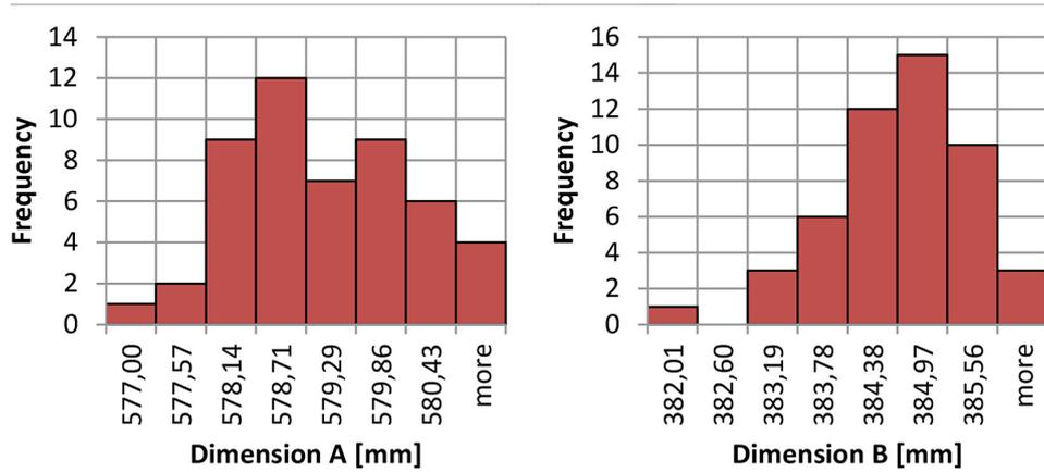
Figure 9. Histogram of dimension A [mm] (left side); dimension B [mm] (right side) – efficiency 15 pcs/min (cardboard packaging No. 2)
