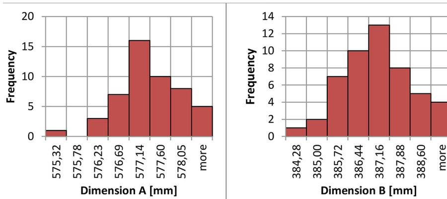
Figure 5. Histogram of dimension A [mm] (left side); dimension B [mm] (right side) – efficiency 15 pcs/min (cardboard packaging No. 1)
