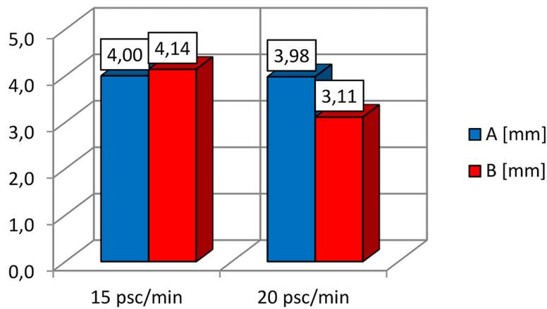
Figure 11. Comparison of the values of dimension A and dimension B divergence in relation to performance for the cardboard packaging No. 2
