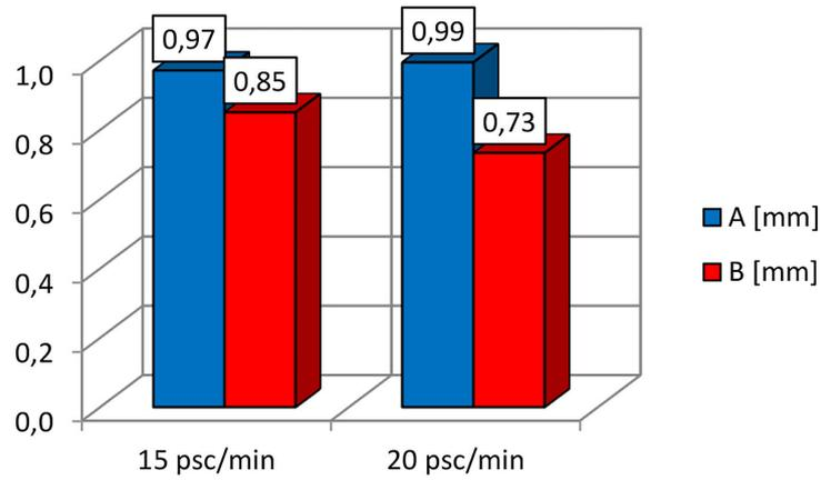
**Figure 12.** Comparison of the standard deviation values of dimension A and dimension B depending on the performance for the cardboard packaging No. 1
