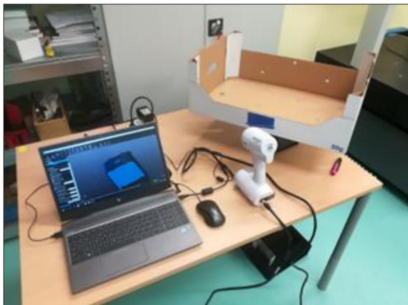
**Figure 1.** Test stand showing Creaform's Academia scanner with the test object
