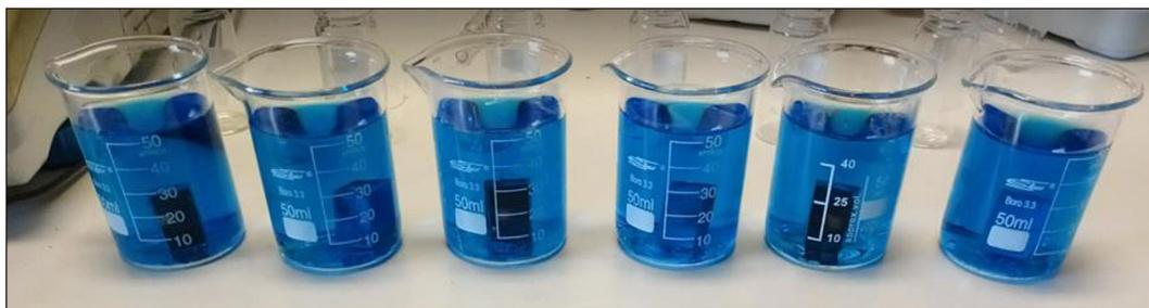
**Figure 2.** Autocatalytic metallization - the last stage in which the tested samples are placed in a metallizing bath
