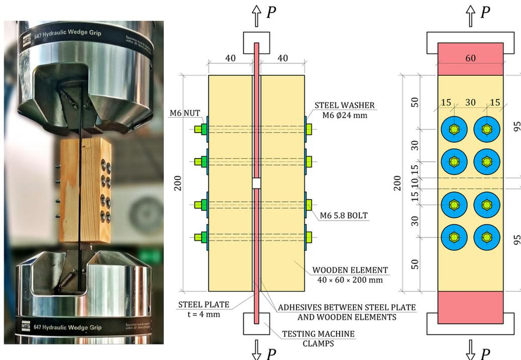
**Figure 1.** Experimental setup: laboratory testing stand and described testing scheme – front and side view (dimensions in mm)
