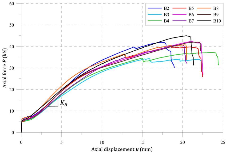
Figure 3. Force-displacement paths for no-adhesive specimens
