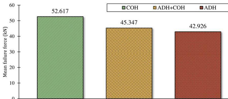
**Figure 8.** Mean failure force depending on the form of failure
