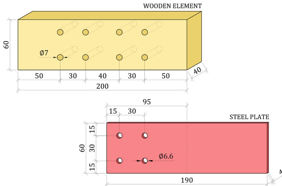
**Figure 2.** Openings pattern in wooden element (yellow) and in steel plate (red) – dimensions in mm
