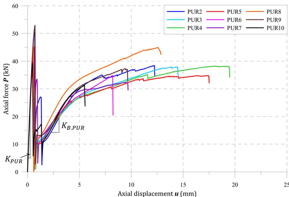
Figure 4. Force-displacement paths for hybrid specimens adhesively bonded with PUR adhesive
