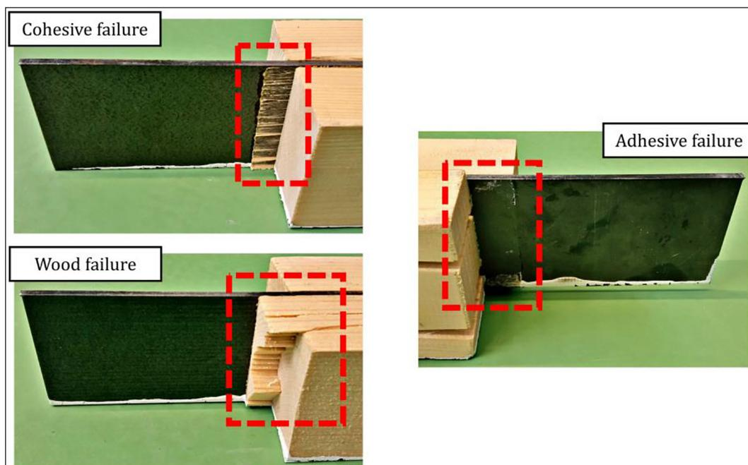
Figure 7. Forms of failure of PUR and PVAc specimens
