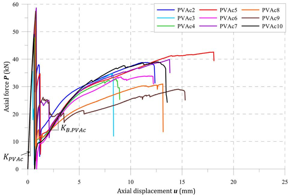
**Figure 5.** Force-displacement paths for hybrid specimens adhesively bonded with PVAc adhesive
