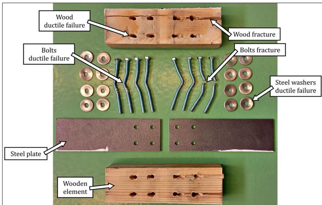
**Figure 6.** Forms of failure of B reference specimens
