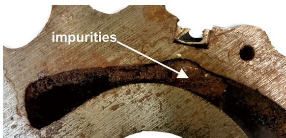
Figure 11. Uncovered cooling conduit in the engine head, partially filled with a mixture of swarf and rust
