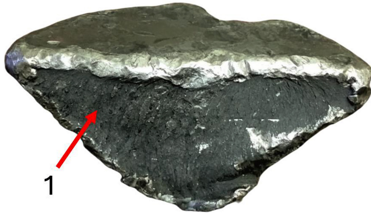
Figure 6. A photograph showing the fracture of the head of the valve no. 2:1 – the fracture is characterized by significant roughness; its shape indicates significant plastic deformation, which is characteristic of acute fractures
