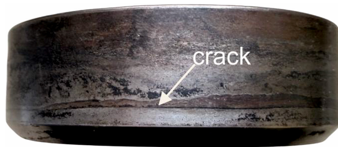
Figure 8. The seat of the exhaust valve no. 1 after having been extracted from the engine head
