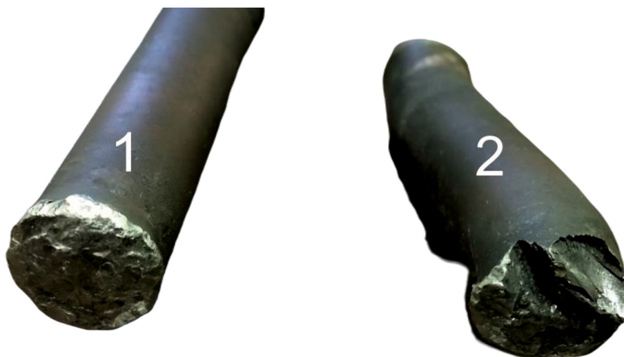
Figure 4. Fractures of the pins of valves no. 1 and 2
