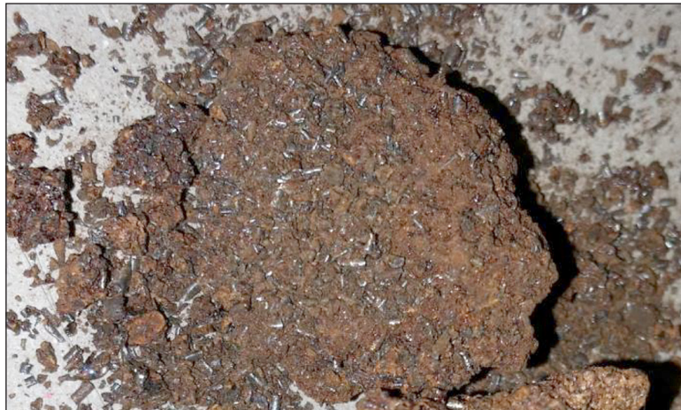
Figure 12. A lump of swarf and rust extracted from the cooling conduit in the engine head
