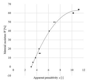
**Figure 3.** Calibration model developed for sensor A and examined aerated concrete
