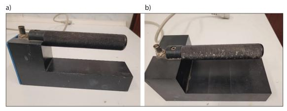
Figure 1. TDR sensors used in experiment (a) Sensor A, (b) Sensor B
