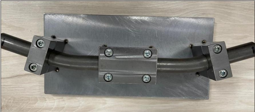
Figure 11. Verification of the geometry of the bent pipe in the device
