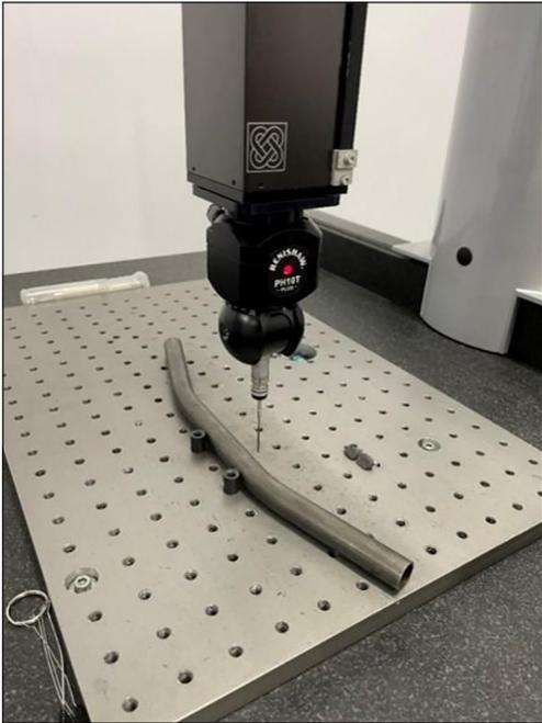
Figure 12. Measurement of pipe geometry on a CMM measuring machine
