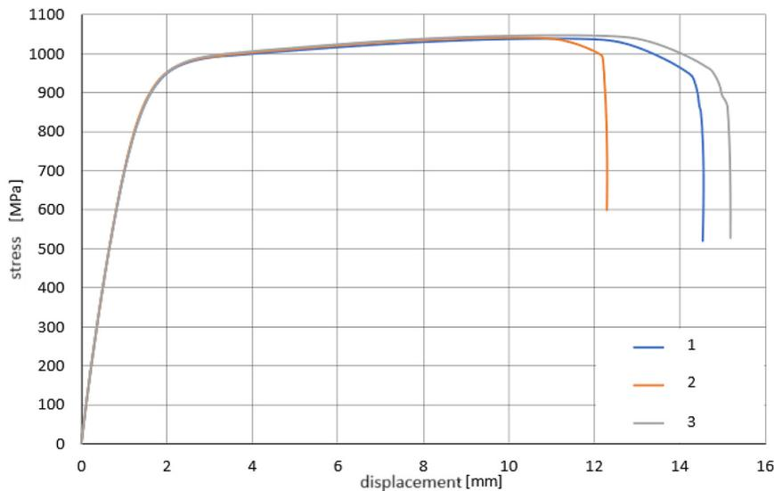
Figure 1. Uniaxial tension diagram of a sample made of steel 1.7734.5
