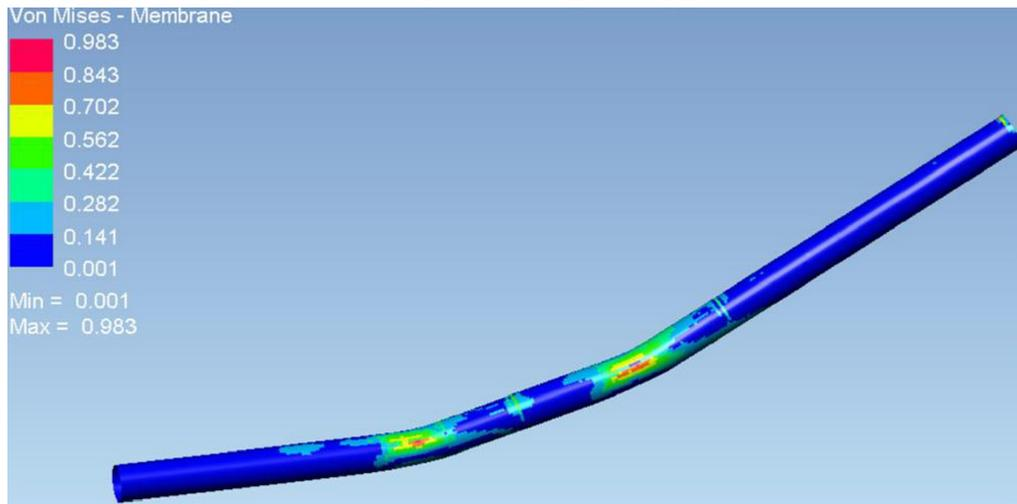
**Figure 6.** Stresses calculated according to the HMH Hypothesis as determined by incremental solver simulation [GPa]
