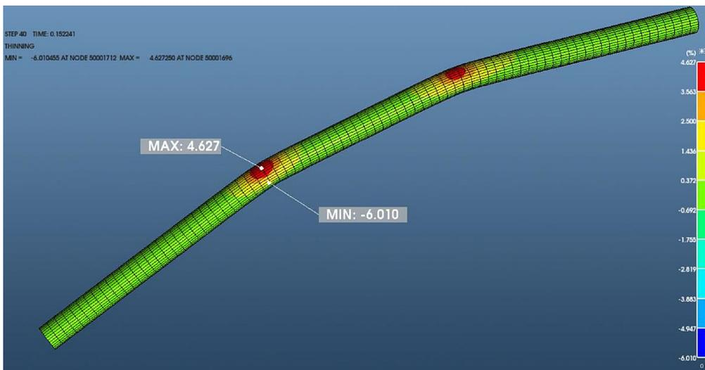
Figure 4. Pipe wall thickness expressed in mm from the outside, as determined by incremental solver simulation
