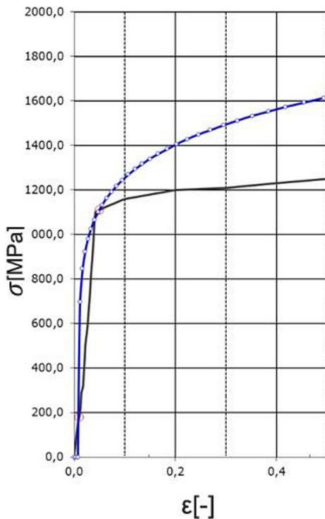
Figure 2. Strengthening curve determined using the Krupowsky-Gesetz method for steel 1.7734.5
