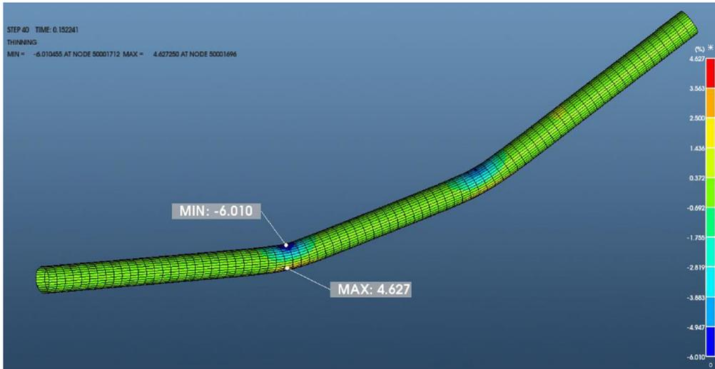
Figure 3. Pipe wall thickness on the inside expressed in mm, as determined by incremental solver simulation
