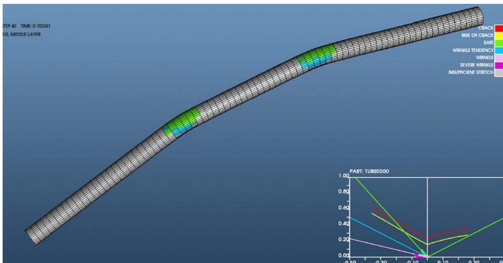
**Figure 7.** FLD curve as determined by incremental solver simulation
