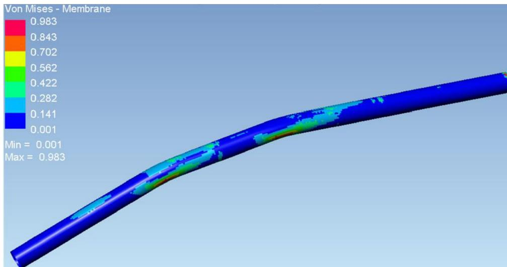
Figure 5. Stresses calculated according to the HMM hypothesis as determined by incremental solver simulation [GPa]
