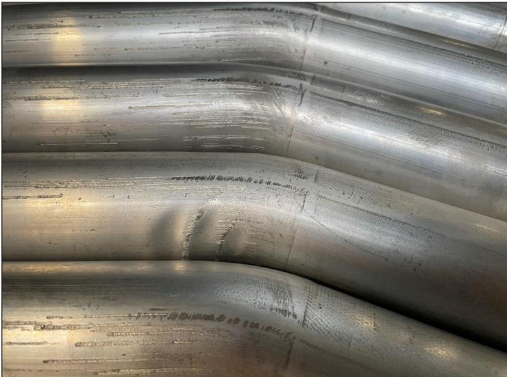
Figure 10. Forming defects in the form of folds of the inner radius
