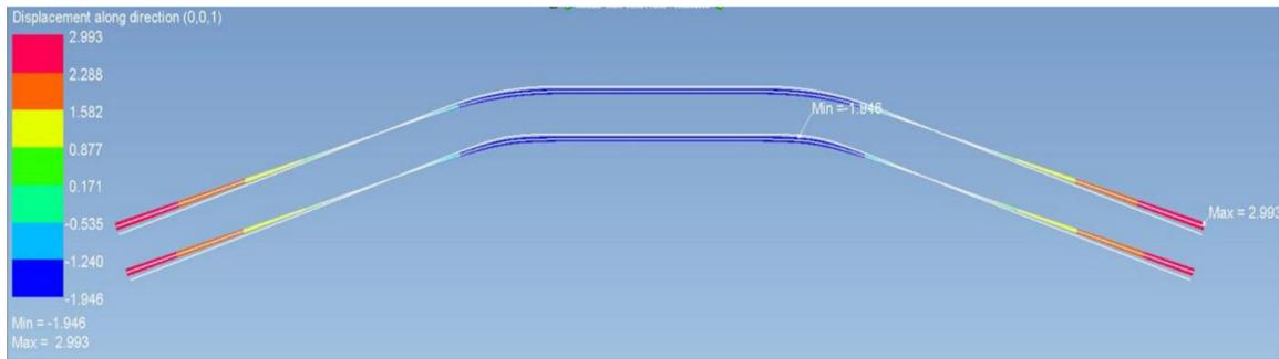
Figure 8. Springback as determined by incremental solver simulation
