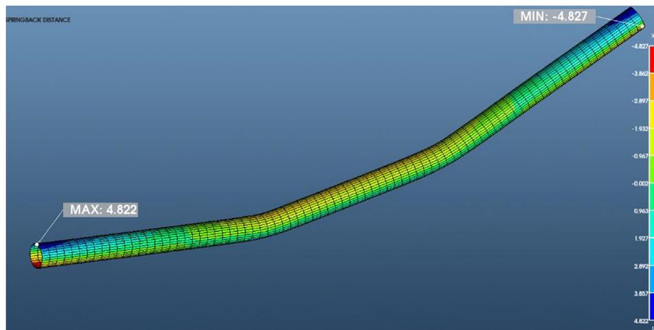
Figure 9. Springback as determined by one step solver simulation
