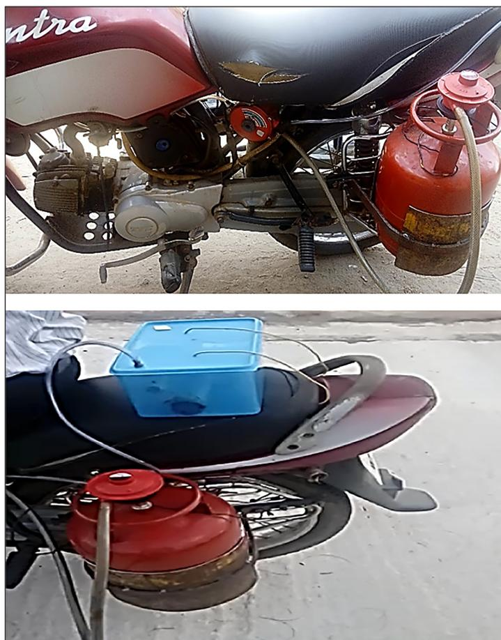
**Figure 9.** Fabricated model of bike which uses LPG + H<sub>2</sub> as fuel
