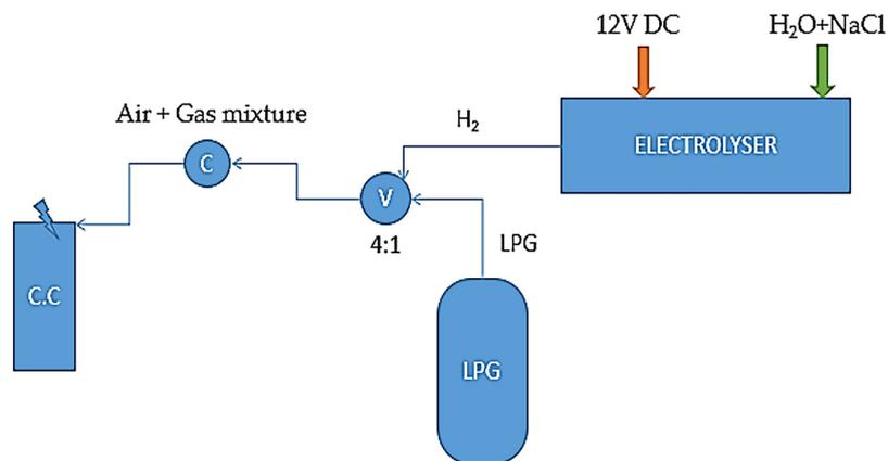
Figure 3. Layout of the experimental setup
