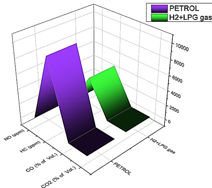
Figure 8. Emission test results between Petrol and H<sub>2</sub> + LPG
