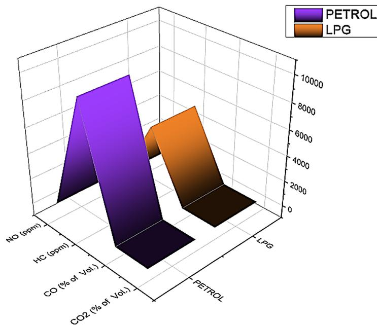
Figure 7. Emission test results between petrol and LPG
