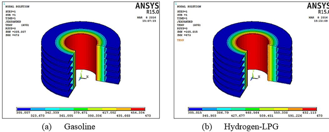
Figure 5. Temperature distribution on the engine cylinder wall
