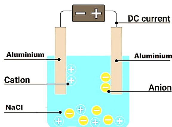
Figure 1. Electrolysis setup
