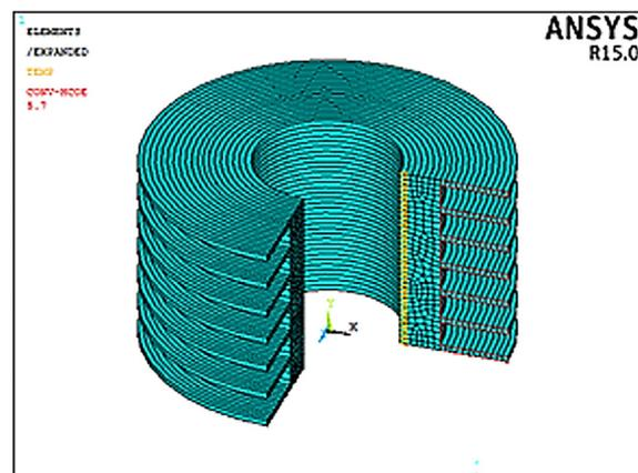
Figure 4. Isometric view of the FE model with fins
