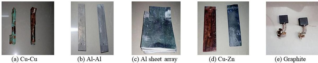
Figure 2. Tested electrodes
