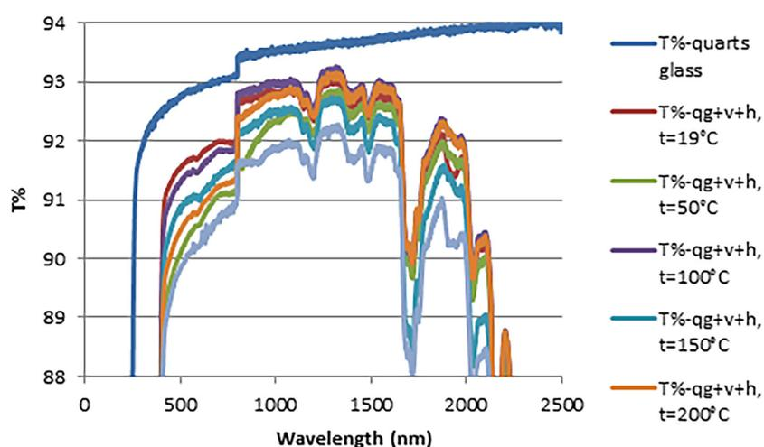
**Figure 7.** Study on the impact of ambient temperature on the light transmittance of clear varnish with hardener, transmittance range from 88% to 94%
