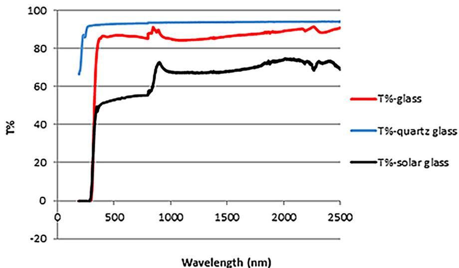
Figure 2. Comparison of light transmittance of glass, quartz glass, and solar glass
