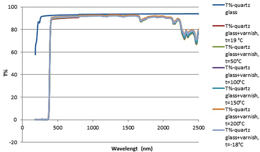
Figure 4. Study on the impact of ambient temperature on the light transmittance of clear varnish without hardener
