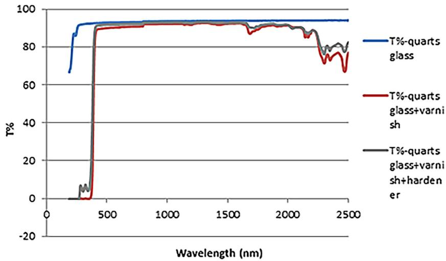
Figure 3. The effect of varnish coating and hardener on the light transmittance of a quartz glass substrate
