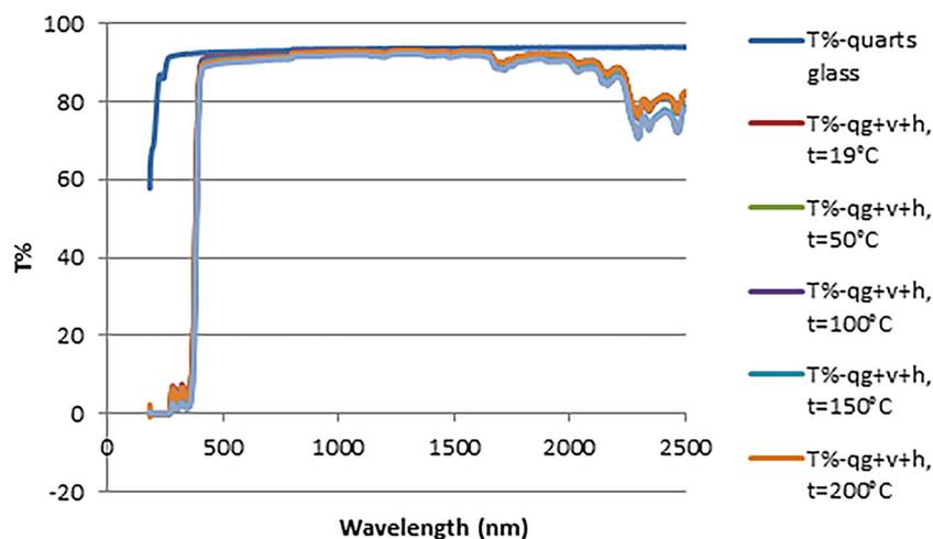
**Figure 6.** Study on the impact of ambient temperature on the light transmittance of clear varnish with hardener
