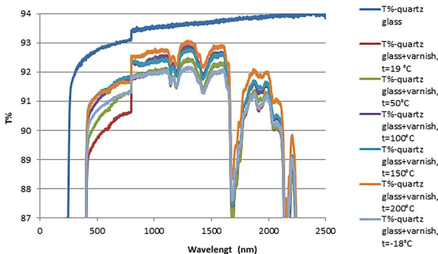
Figure 5. Study of the effect of ambient temperature on the light transmittance of clear varnish without hardener, transmittance range from 87% to 94%
