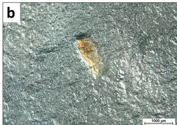
**Figure 4.** Surface microstructure of films with psyllium additives: a) psyllium flour – TPS/PF, and b) psyllium husk – TPS/PH
