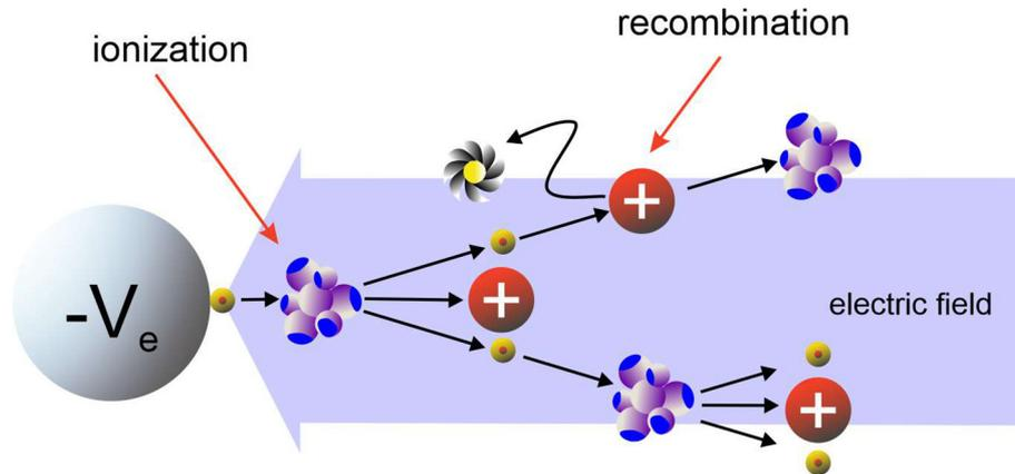
Fig. 12. The mechanism of corona discharge [33, 34]
