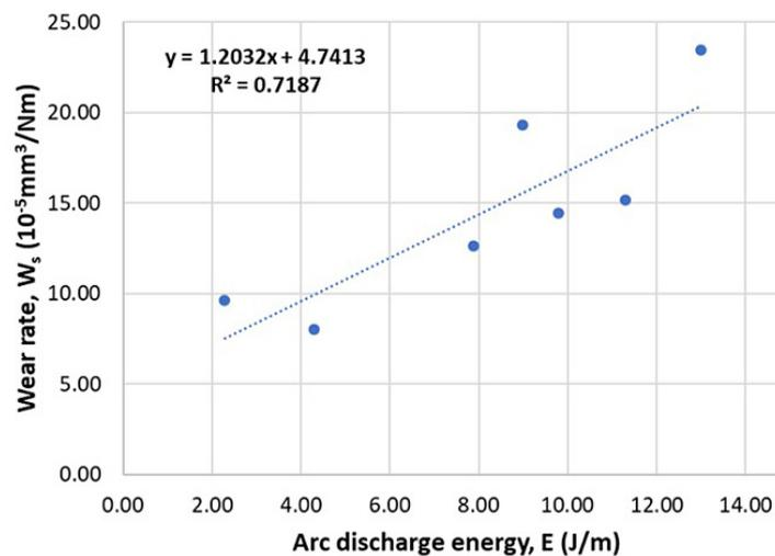
Fig. 9. Strip wear rate compared to arc discharge energy throughout the test
