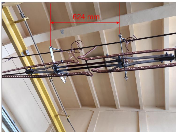
Fig. 3. Bottom view of the section insulator; placed outside, there are guides made of Cu-ETP copper
