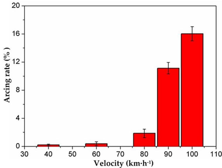
Fig. 10. Electric arc rate of the pure carbon strip in relation to the occurred velocity [27]
