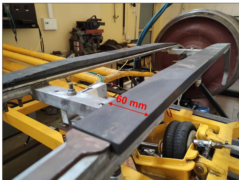
**Fig. 1.** A fragment of the current collector with a visible graphite cap
