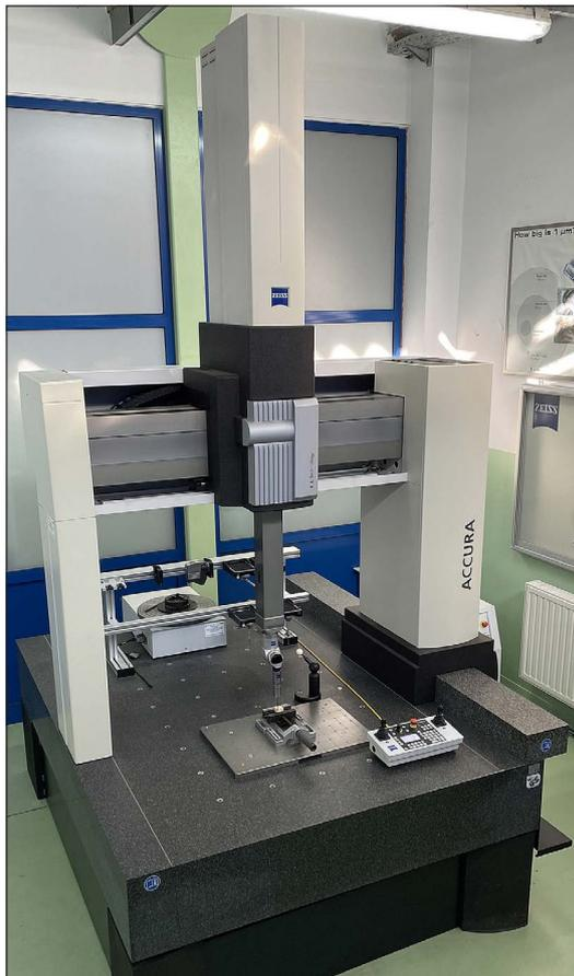
**Fig. 9.** The applied CMM – ACCURA II
