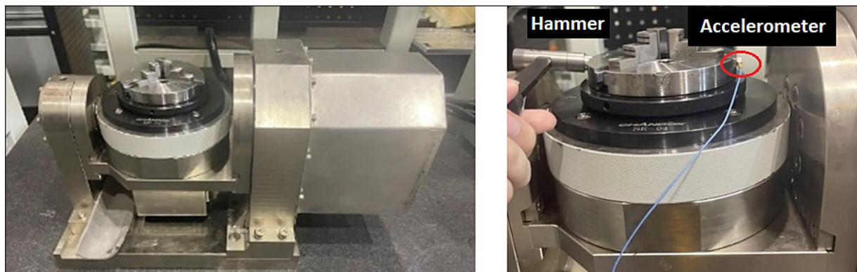
**Fig. 3.** Configuration of tapping test of swivel table placed on the granite platform
