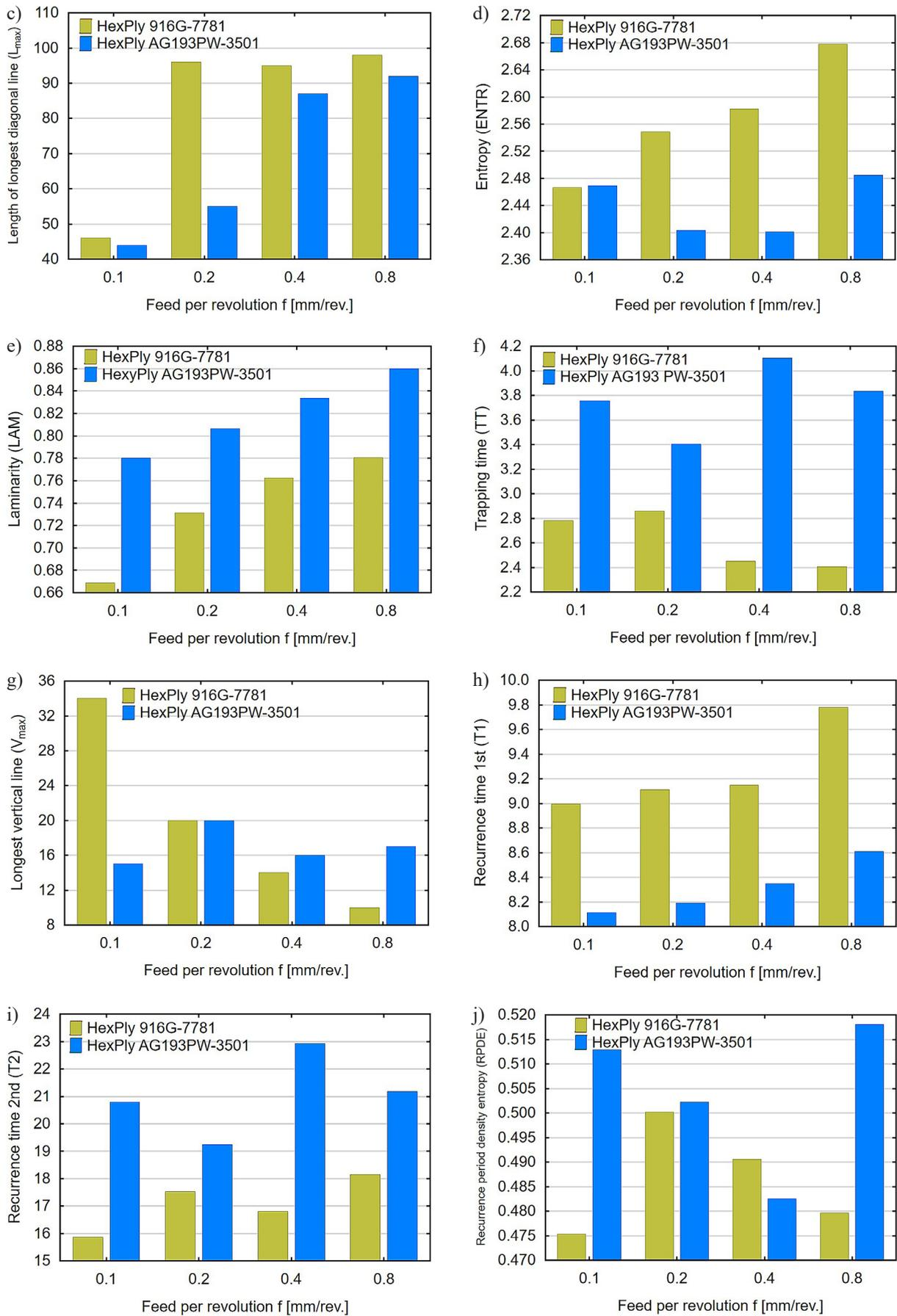
**Fig. 8. Cont.** Influence of feed per revolution on recurrence quantifications: (c)  $L_{max}$ , (d) ENTR, (e) LAM, (f) TT, (g)  $V_{max}$ , (h) T1, (i) T2, (j) RPDE
