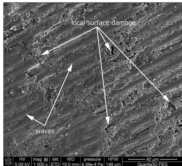
Fig. 4. SEM image obtained after milling for a sample made of CFRP (HexPly AG193PW-3501)
