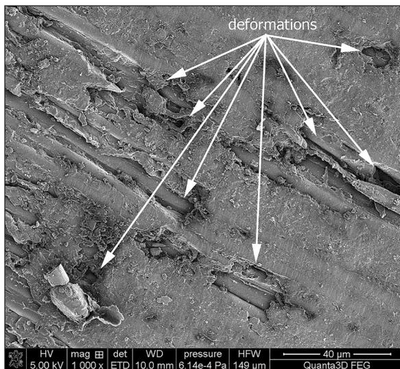
Fig. 3. SEM image obtained after milling for a sample made of GFRP (HexPly 916G-7781)
