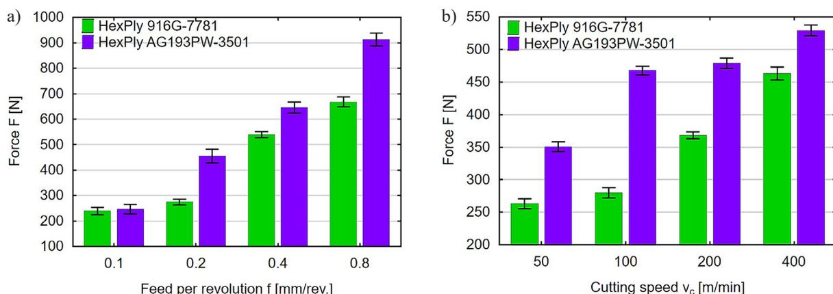
**Fig. 5.** Influence of a) feed per revolution in milling and (b) cutting speed for HexPly 916G-7781 and HexPly AG193PW-3501 on feed force
