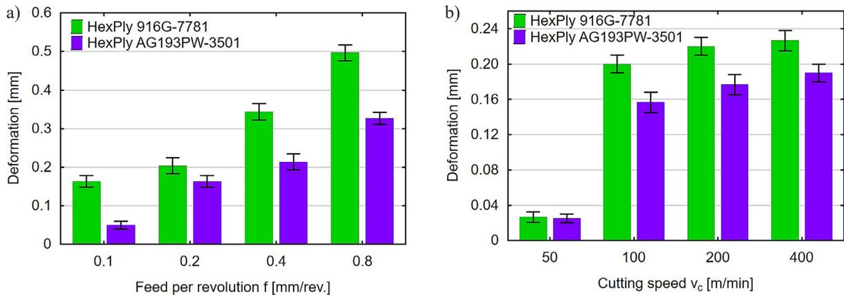
Fig. 6. Influence of a) feed per revolution in milling and (b) cutting speed for HexPly 916G-7781 and HexPly AG193PW-3501 on deformation
