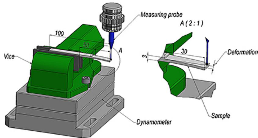
Fig. 2. Scheme of performing deformation measurement
