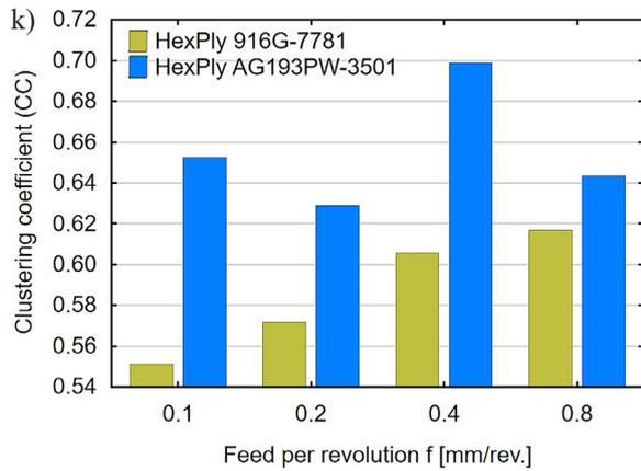
**Fig. 8. Cont.** Influence of feed per revolution on recurrence quantifications: (k) CC
