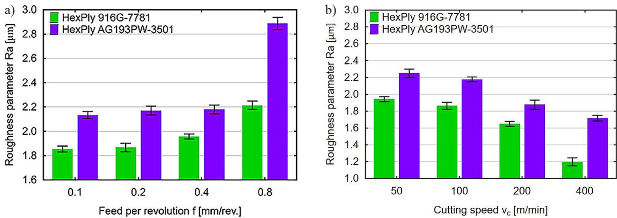
Fig. 7. Influence of a) feed per revolution in milling and (b) cutting speed for HexPly 916G-7781 and HexPly AG193PW-3501 on roughness parameter
