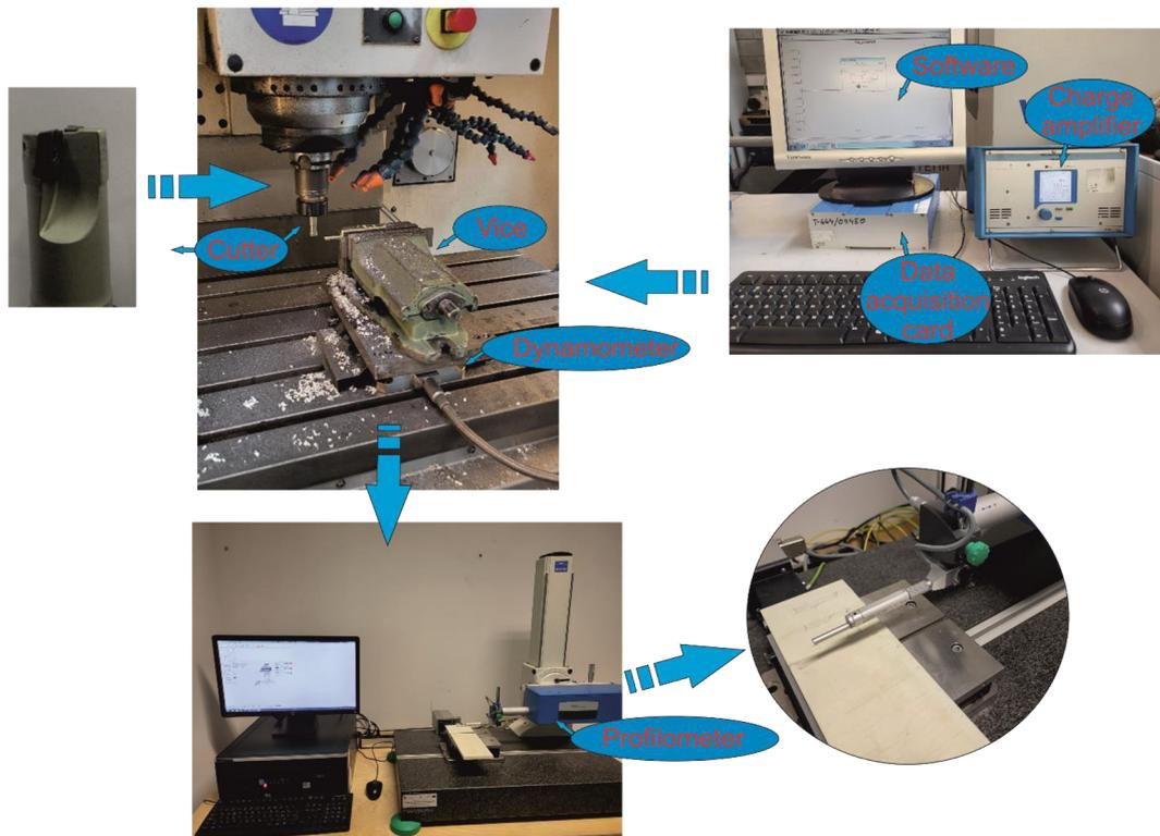
Fig. 1. Scheme of the milling and measuring
