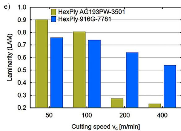
**Fig. 9.** Influence of cutting speed on recurrence quantifications: (a) DET, (b) L, (c)  $L_{\text{max}}$ , (d) ENTR, (e) LAM
