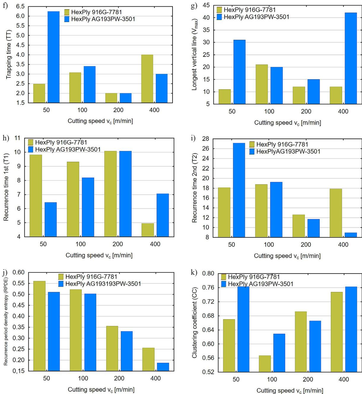
**Fig. 9. Cont.** Influence of cutting speed on recurrence quantifications: (f) TT, (g)  $V_{max}$ , (h) T1, (i) T2, (j) RPDE and (k) CC
