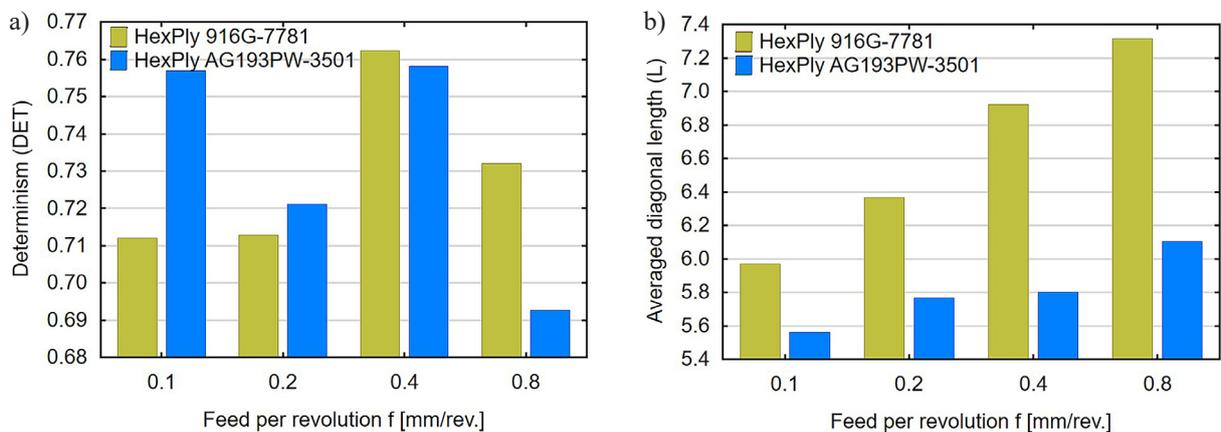
Fig. 8. Influence of feed per revolution on recurrence quantifications: (a) DET, (b) L
